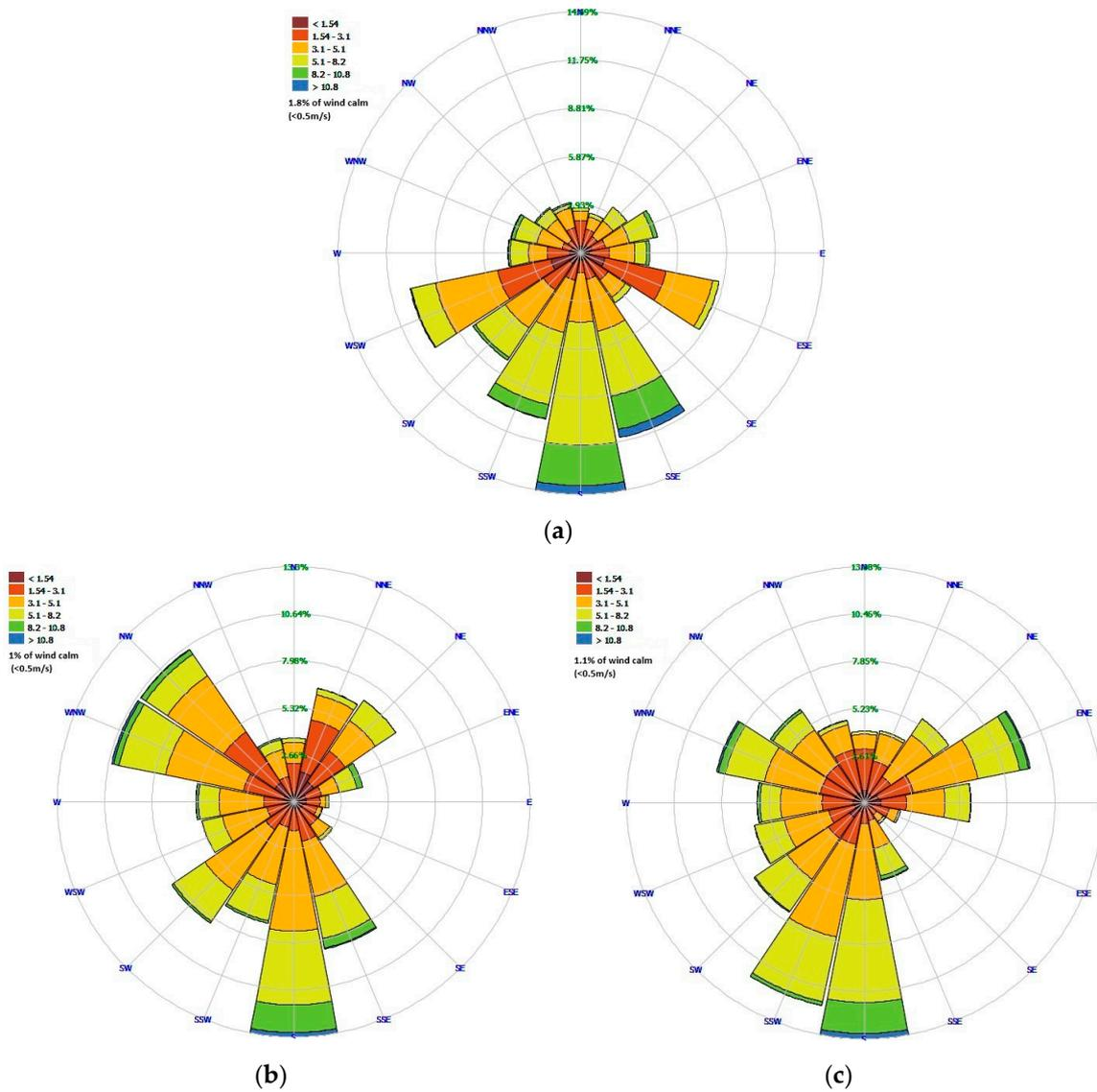
**Figure 8.** The distribution of wind directions and wind speeds determined by the WRF/CALMET model in the meshes of the meteorological grid corresponding to the location of selected towns in 2018 (Source: Own study): (a) Bogatynia, (b) Sieniawka, (c) Działoszyn.
