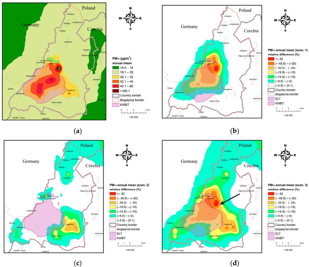
**Figure 16.** Annual mean PM<sub>10</sub> concentrations in 2018: modeled values and relative differences for the analyzed scenarios (source: own study): (a) in 2018, (b) relative difference for scenario 1, (c) relative difference for scenario 2, (d) relative difference for scenario 3.
