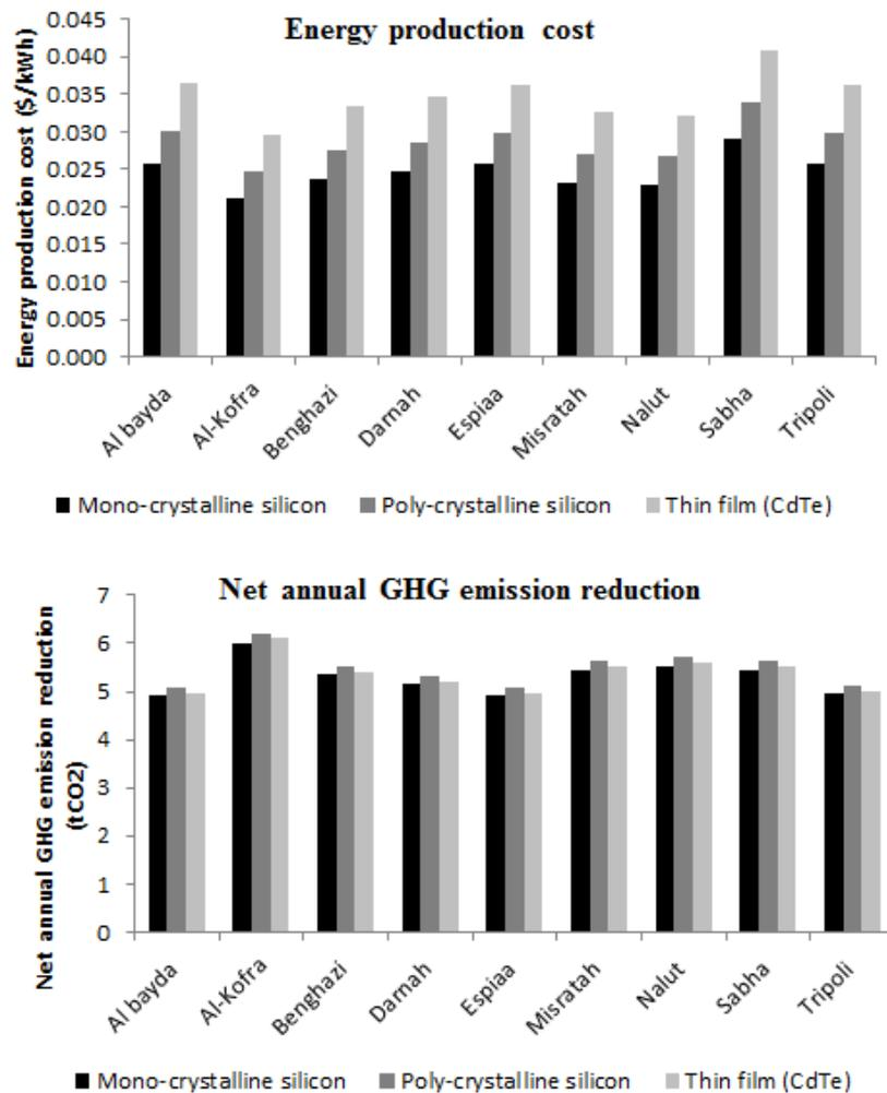
Figure 8. Sensitivity analysis for the 5kW grid-connected solar PV system.
