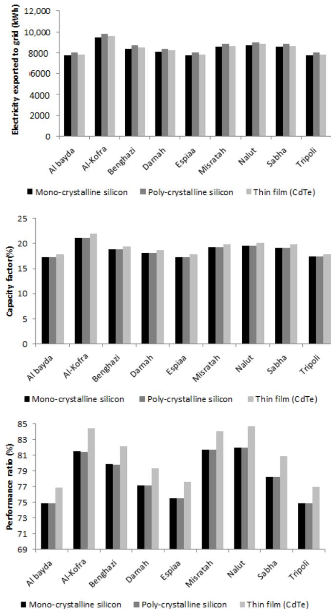
Figure 7. Annual electricity generation, capacity factor, and performance ratio of the proposed systems.
