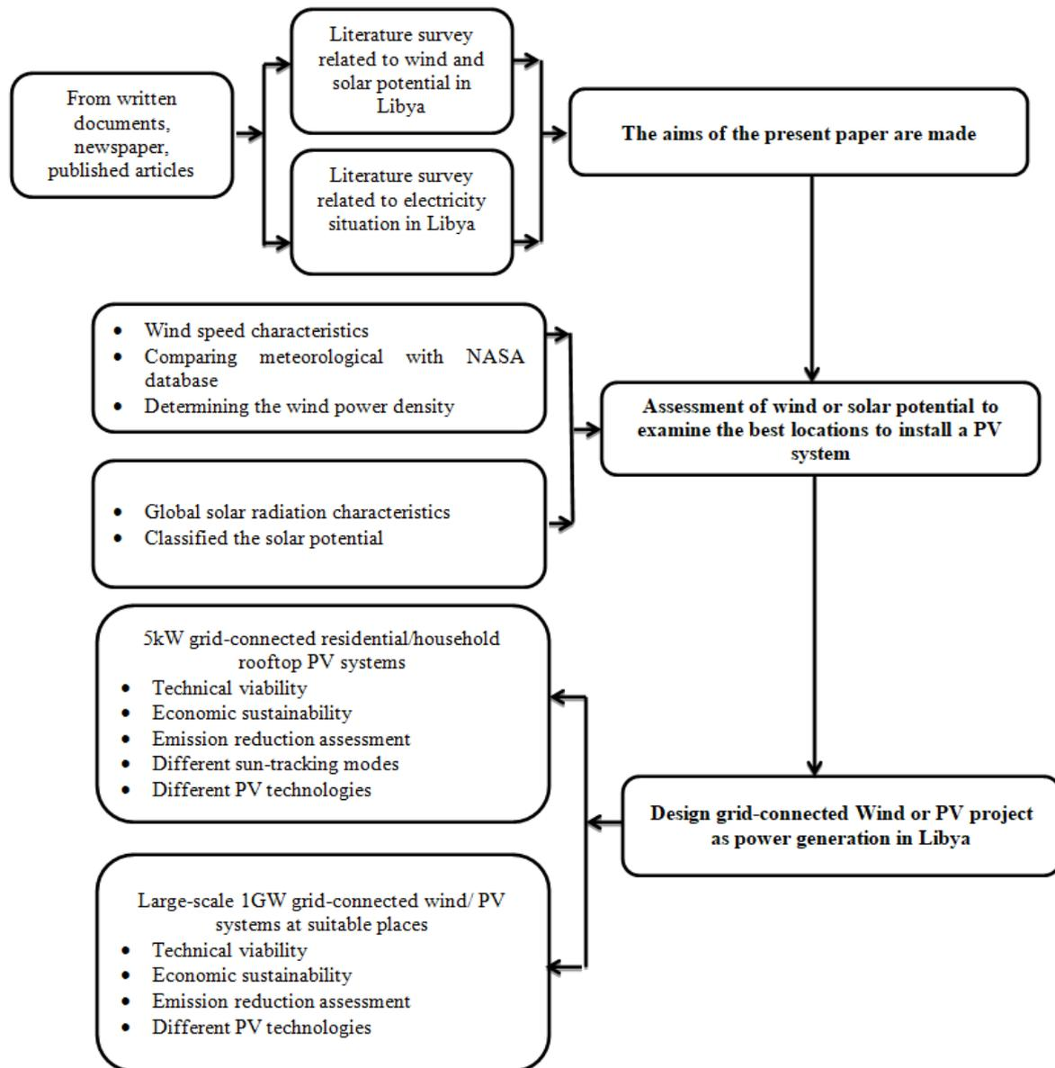
**Figure 1.** Schematic description for the proposed methodology.
