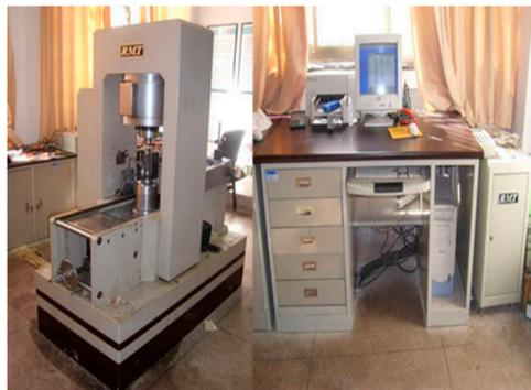
**Figure 3.** RMT-150B servo-control testing machine.
