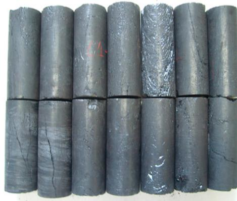
**Figure 2.** Coal samples as prepared for experiment.
