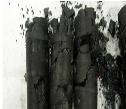
**Figure 5.** Failure pattern of coal samples.
