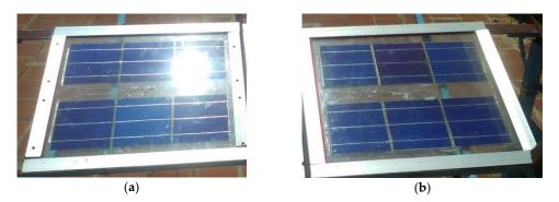
Figure 3. Photographic view: (a) STPV module without PCM; (b) STPV module with PCM.
