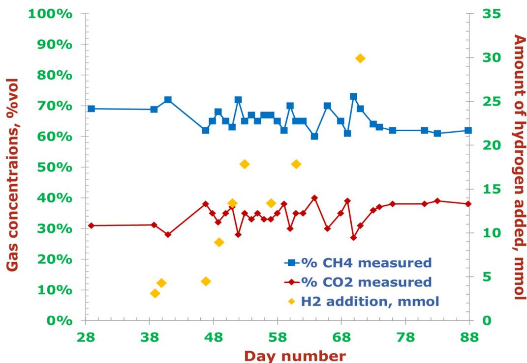
**Figure 2.** Effect of H<sub>2</sub> injection on biogas composition (*v/v*) in terms of standard temperature and pressure (STP) normalized CH<sub>4</sub> and CO<sub>2</sub> contents.
