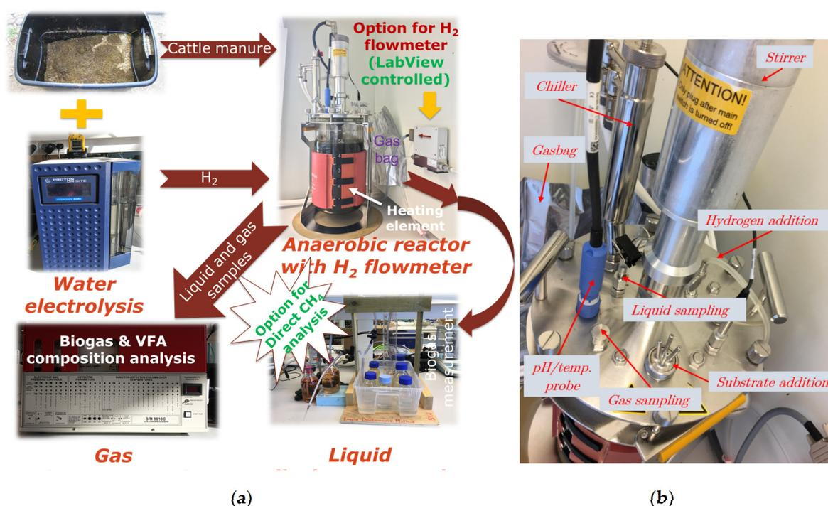
**Figure 1.** Experimental set-up: (a) different processing steps; (b) top view of the reactor Biostat<sup>®</sup> A showing location of different ports and sensors.
