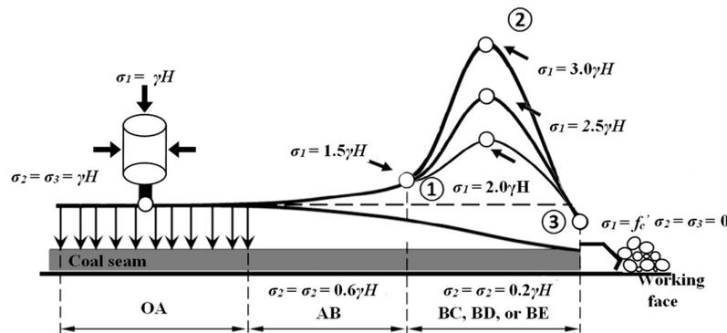
Figure 4. The stress state of coal mass in front of the working faces under three different mining layouts.
