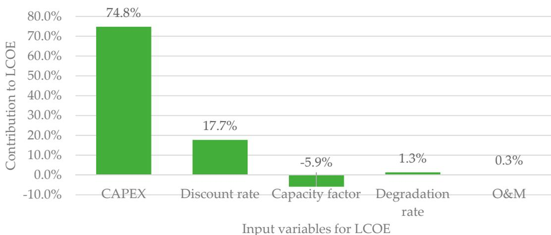
**Figure 13.** Sensitivity of the residential solar LCOE.
