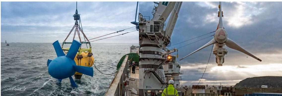
**Figure 1.** Sabella D10 (left) and Atlantis AR1500 tidal stream turbines (TSTs; right) [15].
