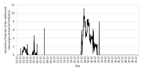
**Figure 11.** Flowrate of natural gas required to supplement the gas from methane drainage to reach a concentration of 40% in December.
