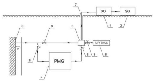
**Figure 14.** Diagram of technology for the stabilization of parameters of gas captured from methane drainage with the use of underground tanks: 1—methane drainage station; 2—gas engines; 3—mixer; 4—methane tank; 5—air tank; 6—operation area; 7—pipeline; 8—valves with PMG sensors, underground gas tank; SO—methane capture station; SG—gas engine station [37].
