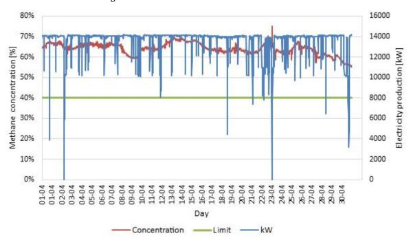
Figure 5. Methane concentration and electricity production in April.
