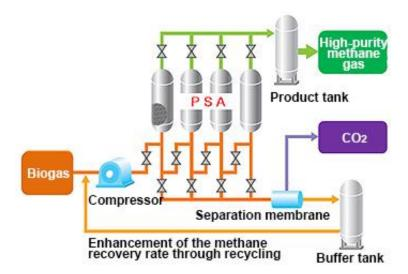
**Figure 13.** Diagram of a hybrid biogas purifying installation with the use of PSA technology and membrane separation [35].
