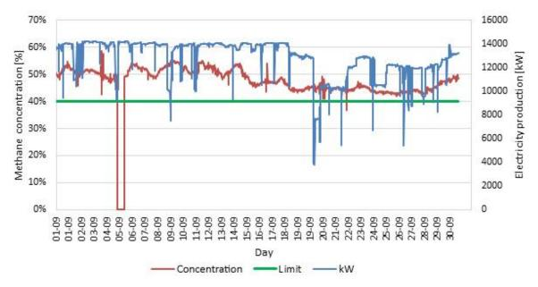
Figure 7. Methane concentration and electricity production in September.
