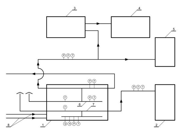
**Figure 1.** Flow chart of methane utilization: 1—methane drainage station; 2—compressor hall; 3—reduction station; 4—heat and power plant; 5—gas engines; 6—pressure collector II stage; 7—pressure collector I stage; 8—pipeline with methane–air mixture from hard coal mine; F—gas flowrate measurement; H—gas humidity measurement; P—gas pressure measurement; Q—gas quality measurement; T—gas temperature measurement.
