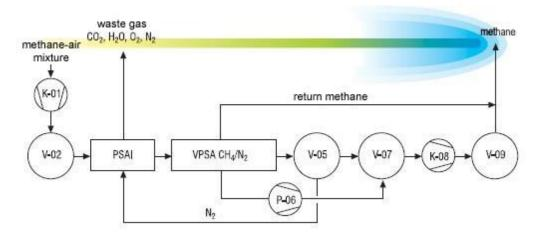
**Figure 12.** Diagram of the methane–air mixture enrichment installation: K-01—gas compressor; V-02—buffer; V-07—CH4 buffer; PSA I—purification PSA module; VPSA CH4/N<sub>2</sub>—methane enrichment PSA module; V-05—N<sub>2</sub> buffer; P-06—vacuum pump; K-08—CH4 compressor; V-09—CH4 buffer [33].
