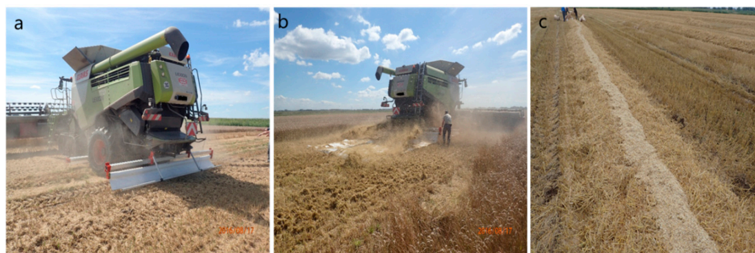
Figure 2. (a) Unrolling sheet installations below the combine harvester and (b) in operation. (c) Chaff placed on the straws.
