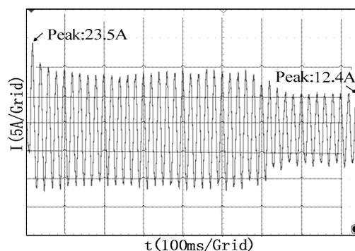
**Figure 18.** Test waveforms of the phase current of the stator winding in asynchronous mode.
