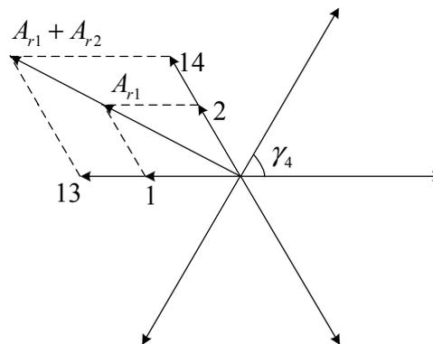
Figure 6. Slot electrical potential star Vectogram ( $p = 4$ ).
