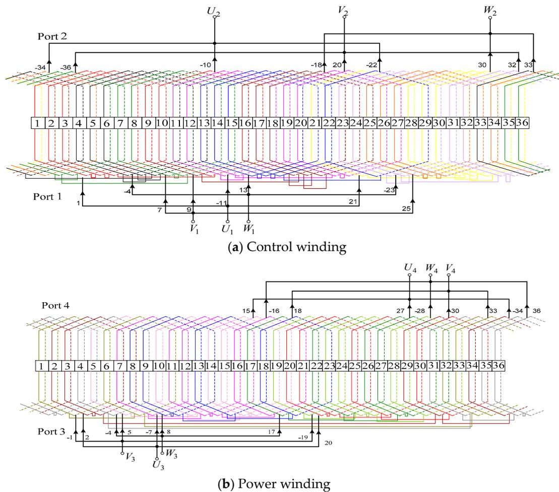
Figure 8. The wiring structure of the stator winding.
