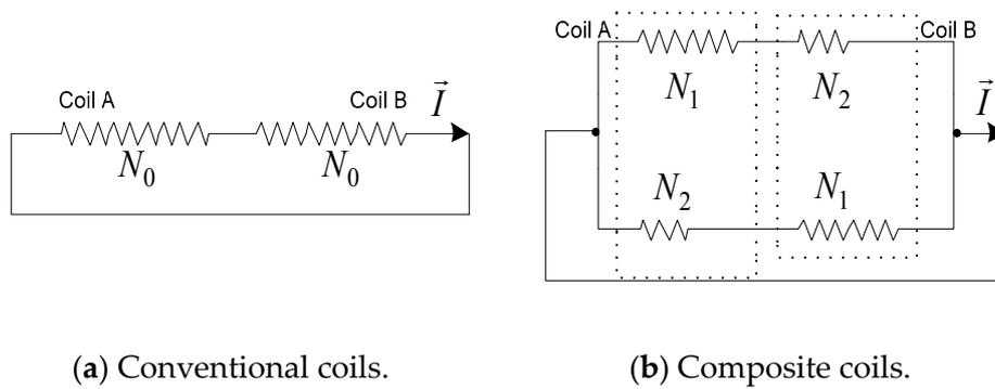
Figure 2. A rotor winding branch composed separately of common coils and composite coils.
