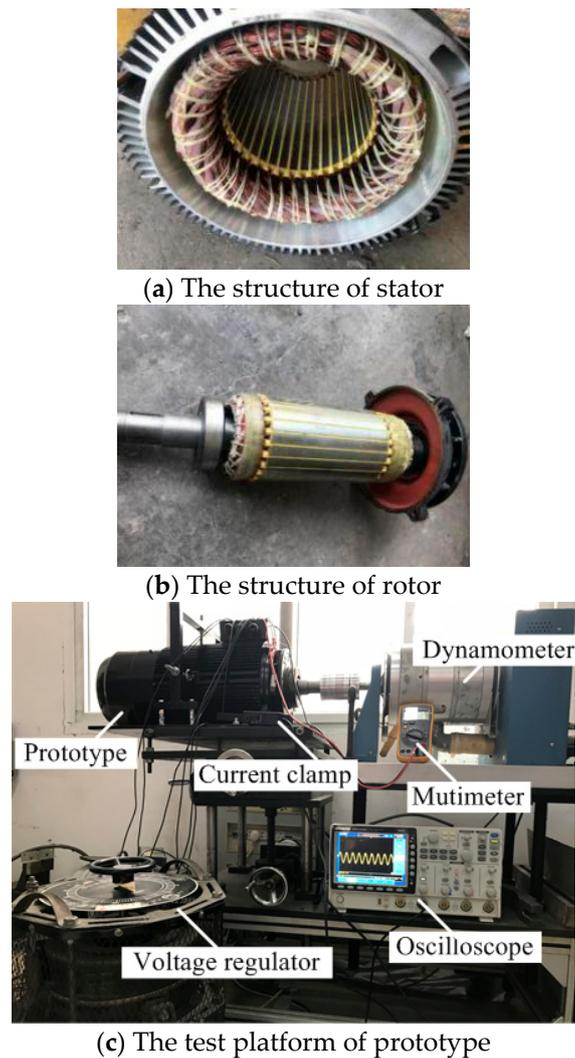
**Figure 11.** Stator, rotor structures, and test platform of the prototype.
