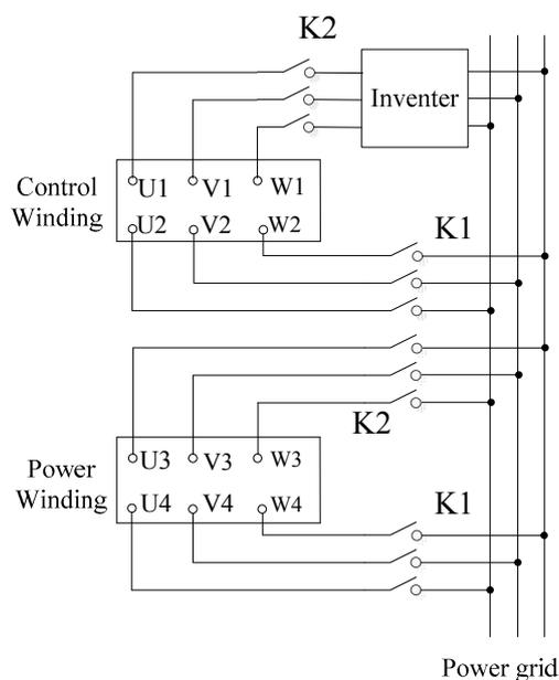
Figure 10. The port wiring diagram of the prototype when it is overall running.
