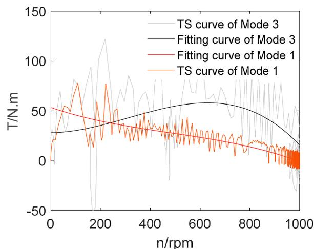
Figure 13. The fitting curve of transient torque-speed.
