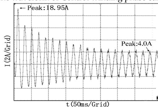
(b) The waveform of the Power winding phase current.
