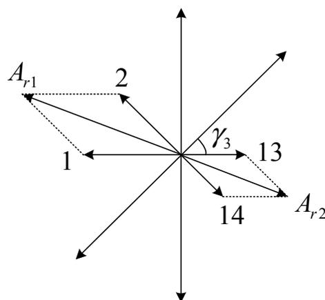
Figure 7. Slot electrical potential star Vectogram ( $p = 3$ ).
