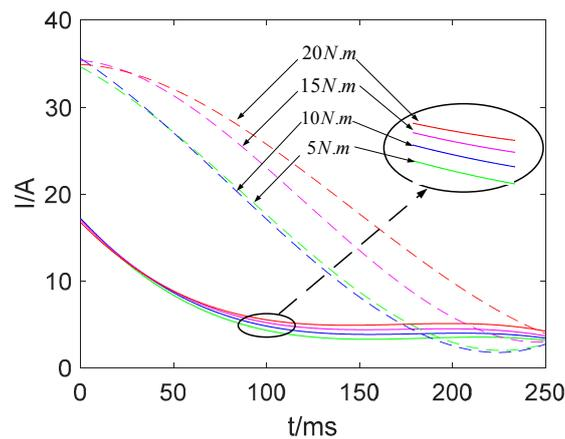
(b) The fitting curve of Power winding (PW).
