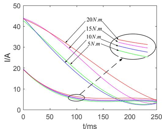
(a) The fitting curve of Control winding (CW).
