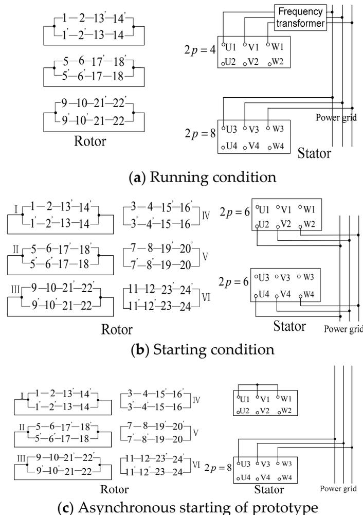
**Figure 9.** Stator and rotor winding wiring diagram under different working conditions.
