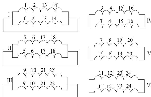
**Figure 5.** The connection of rotor windings.
