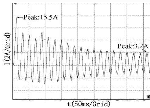
(a) The waveform of Control winding phase current.
