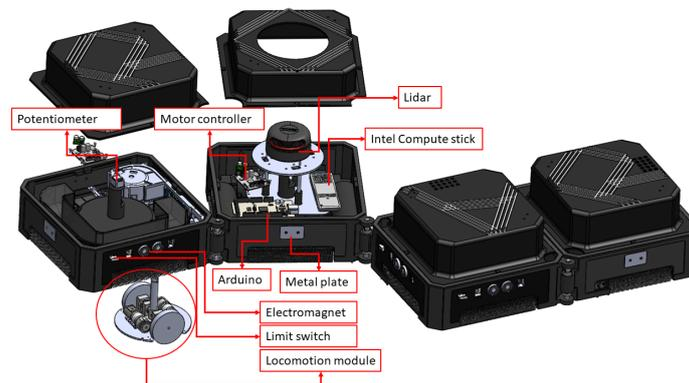
Figure 1. hTetro platform with hardware component setting.
