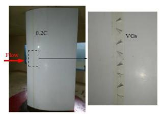
Figure 5. Test airfoil and VG geometric models.
