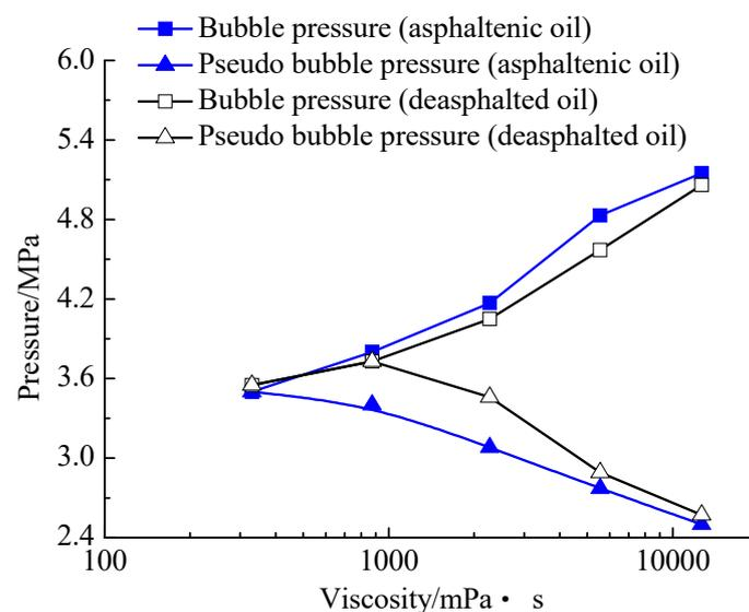
Figure 7. Effect of oil viscosity and asphaltene on bubble pressure and pseudo-bubble pressure.
