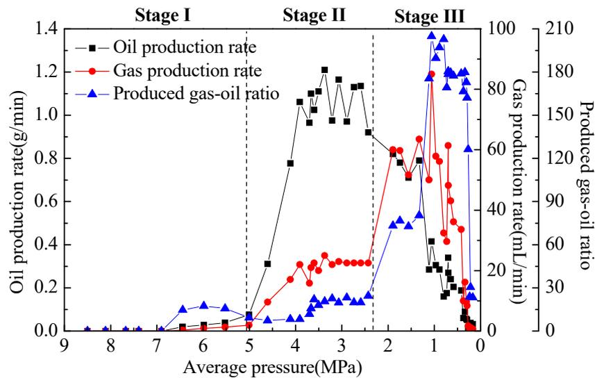
Figure 4. Characteristics for foamy oil depletion development (taking test 1 as an example).
