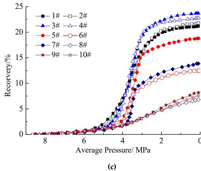
**Figure 3.** Production behavior for the ten depletion experiments. (a) Change in average pressure with time. (b) Change in production gas–oil ratio with average pressure. (c) Change in oil recovery with average pressure.
