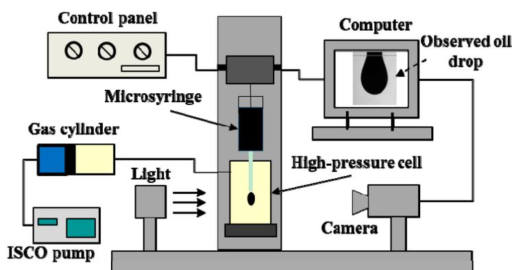
**Figure 2.** Schematic of the pendant drop tensiometer.
