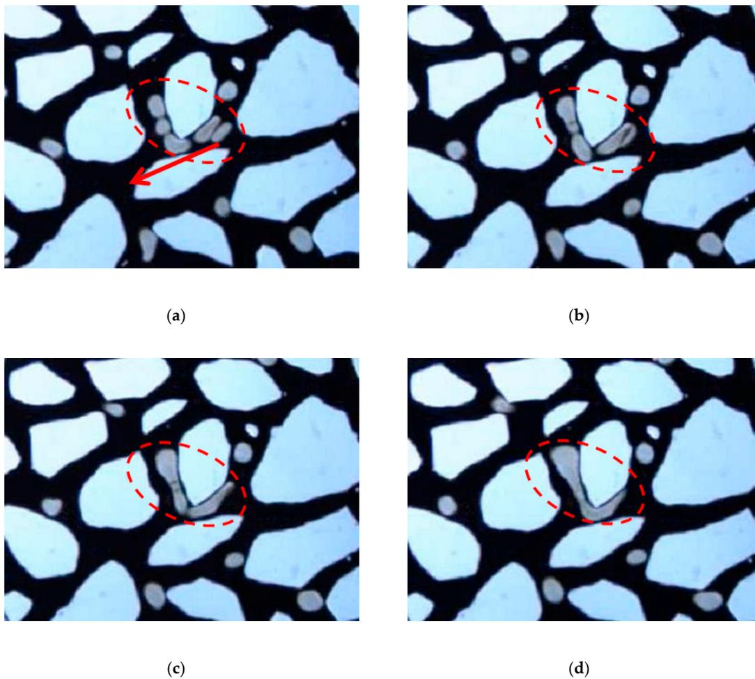
**Figure 11.** A continuous process whereby bubbles coalesce: (a) bubbles come across; (b–d) bubbles coalesce.
