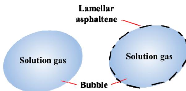
Figure 15. Schematic showing how asphaltene plays a protective role akin to armor on the bubble film.
