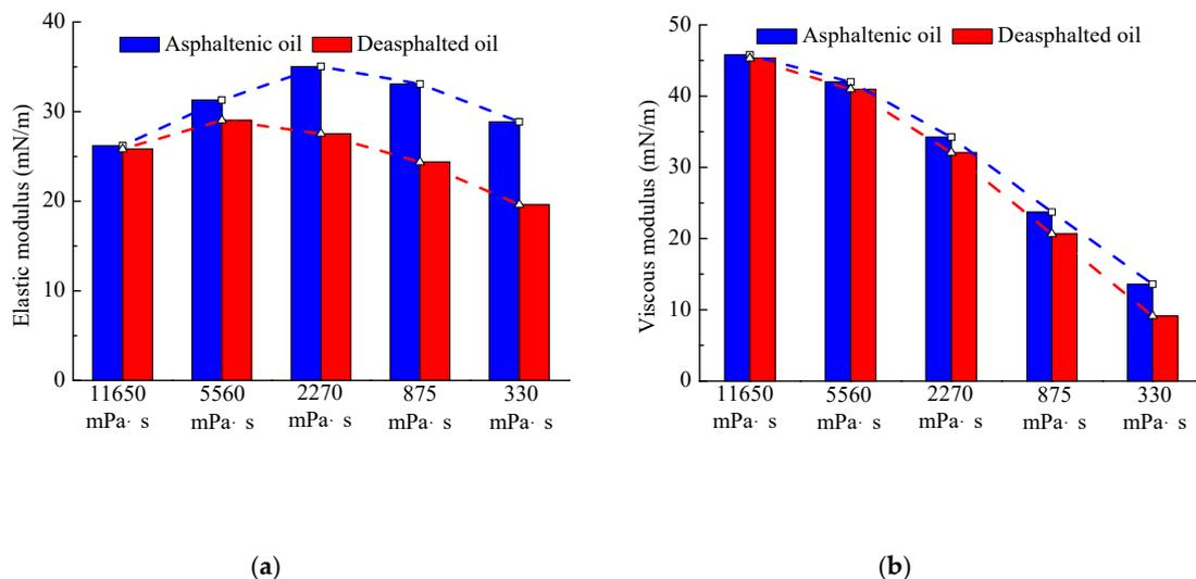
Figure 13. Effect of asphaltene on the elastic modulus and viscous modulus at different viscosities: (a) elastic modulus; (b) viscous modulus.
