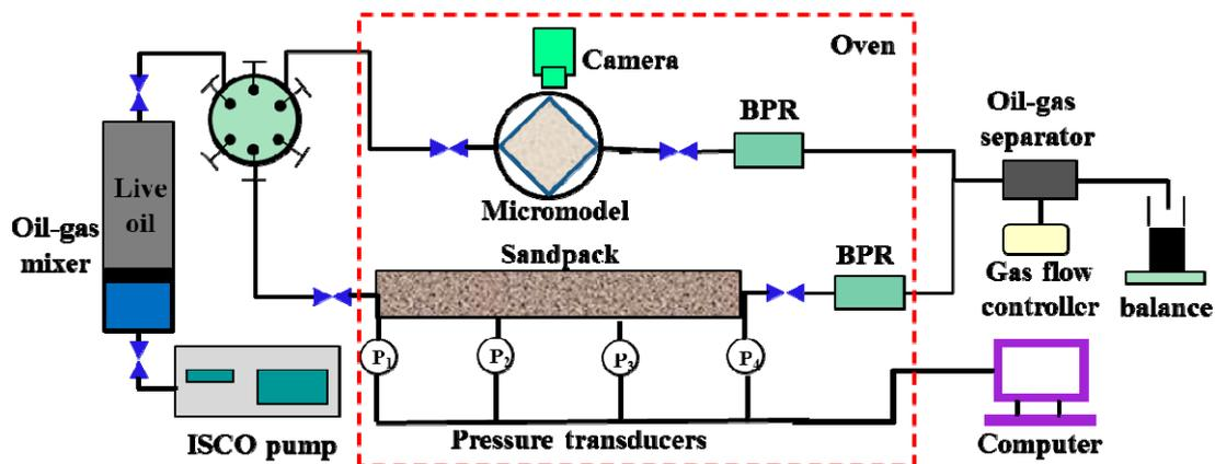
Figure 1. Schematic diagram of depletion experiment in the sandpack and micromodel.
