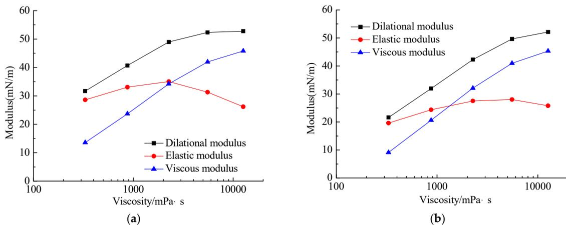
Figure 12. Changes in viscoelastic moduli with viscosity: (a) asphaltenic oil; (b) deasphalted oil.
