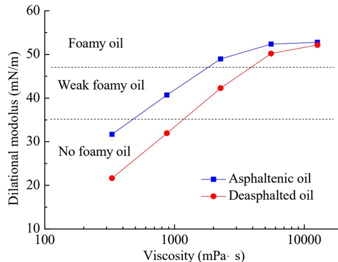
**Figure 14.** Viscoelastic modulus and the performance of depletion experiments of the ten oil samples.
