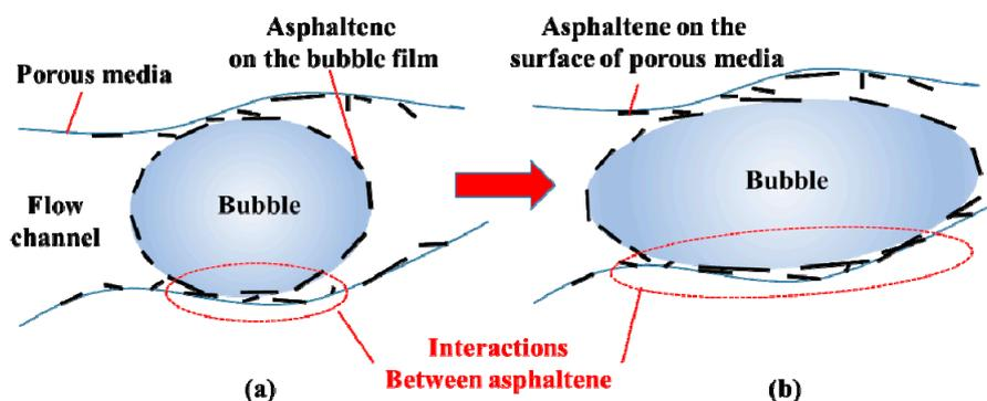
Figure 16. Schematic showing how interactions between the asphaltene on the bubble film and on the surface of porous media promote the bubble to deform and stretch. (a) Interlacement between the asphaltenes on the bubble film and on the surface of porous media; (b) Bubble deformation and stretch happens due to the interlacement.
