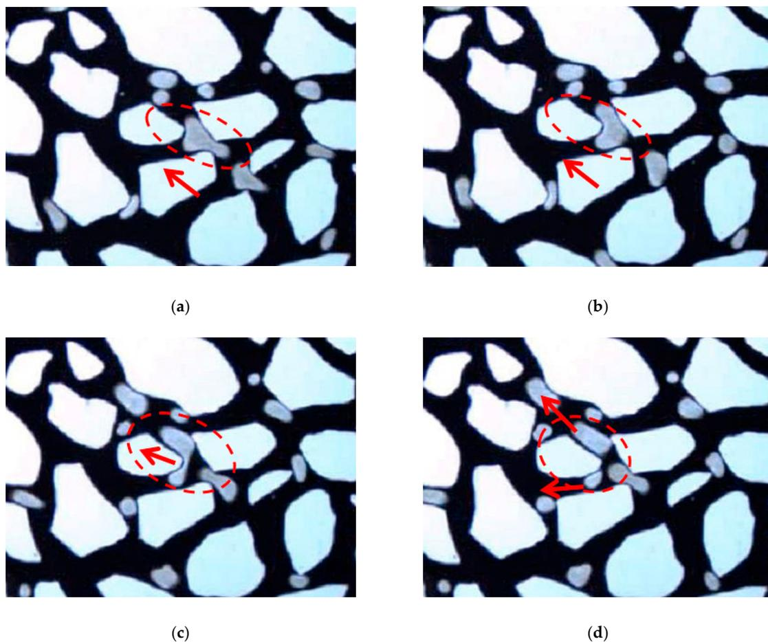
**Figure 10.** A continuous process whereby the bubble goes through a pore throat and then splits into small bubbles: (a) bubble deforms; (b) bubble is elongated; (c) bubble gets thinner; (d) bubble splits.
