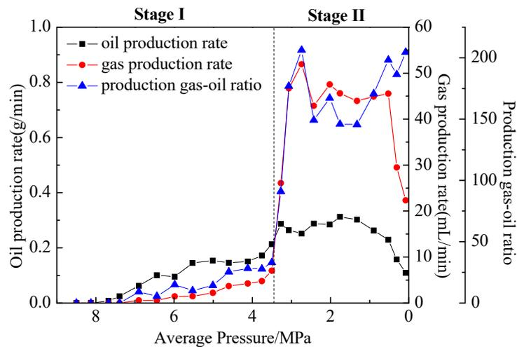
Figure 6. Characteristics for conventional solution gas drive (taking test 8 as an example).
