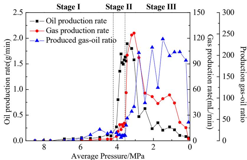
Figure 5. Characteristics for weak foamy oil depletion development (taking test 7 as an example).
