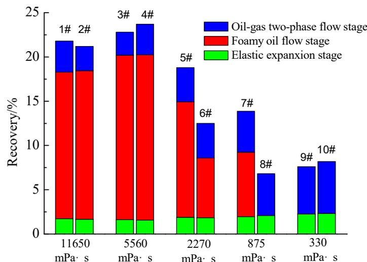
**Figure 8.** Effect of oil viscosity and asphaltene on the total recovery and the recovery of each stage.
