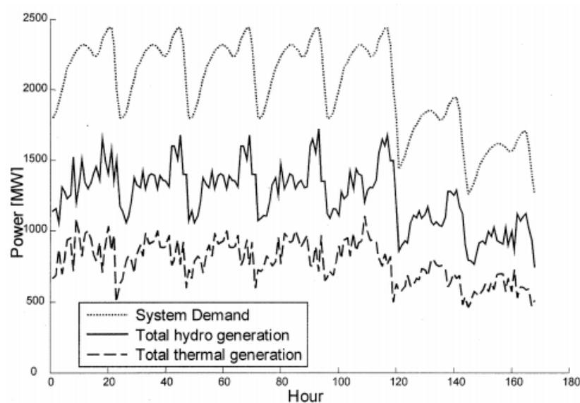
Figure 3. Thermal and hydro generation scheduled for a week.
