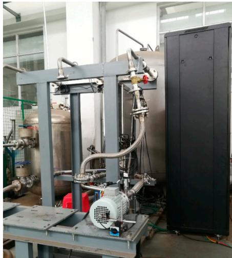
**Figure 7.** Drive pump test bench.
