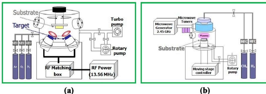
**Figure 1.** Schematic of the (a) RF magnetron sputtering system and (b) MPECVD.
