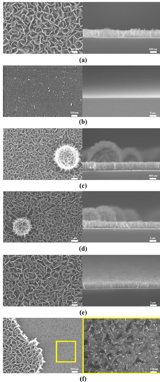
**Figure 2.** FESEM surface (left) and cross-section (right) images of the carbon nanowall (CNW) directly grown on an Si wafer (a) before and (b) after ultrasonic cleaning in acetone; the CNW grown on ITO (c) before and (d) after ultrasonic cleaning in acetone; and the CNW grown on TiN (e) before and (f) after ultrasonic cleaning in acetone.
