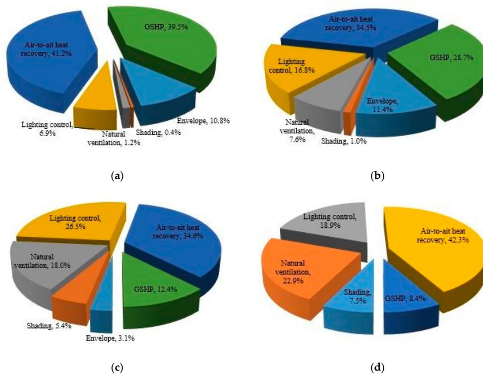
**Figure 18.** The weight of various technologies in four climatic regions. (a) The weight of various technologies in SC region; (b) The weight of various technologies in CC region; (c) The weight of various technologies in HS/CW region; (d) The weight of various technologies in HS/WW region.
