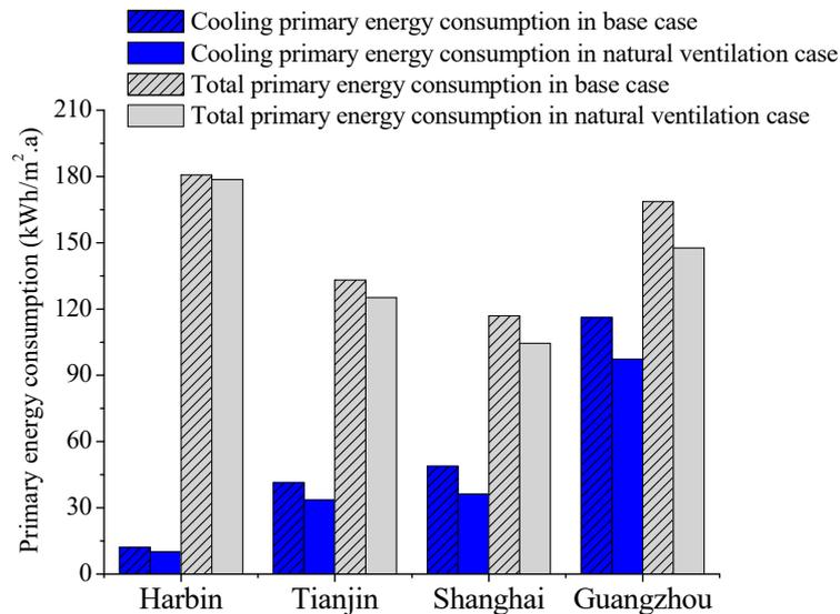
Figure 12. Primary energy consumption in natural ventilation case and base case in four cities.
