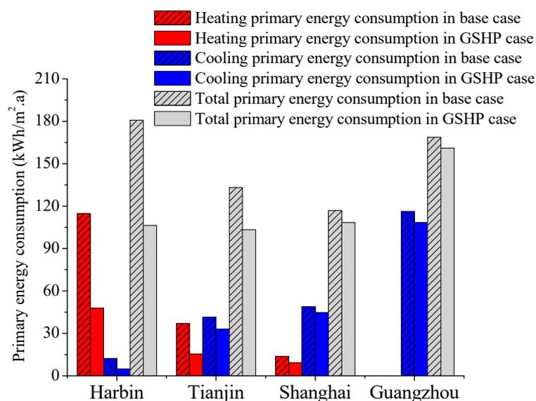
**Figure 17.** The primary energy consumption in GSHP case and base case in four cities.
