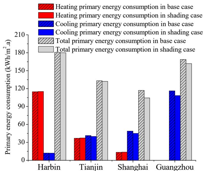
**Figure 10.** Primary energy consumption in shading case and base case in four cities.
