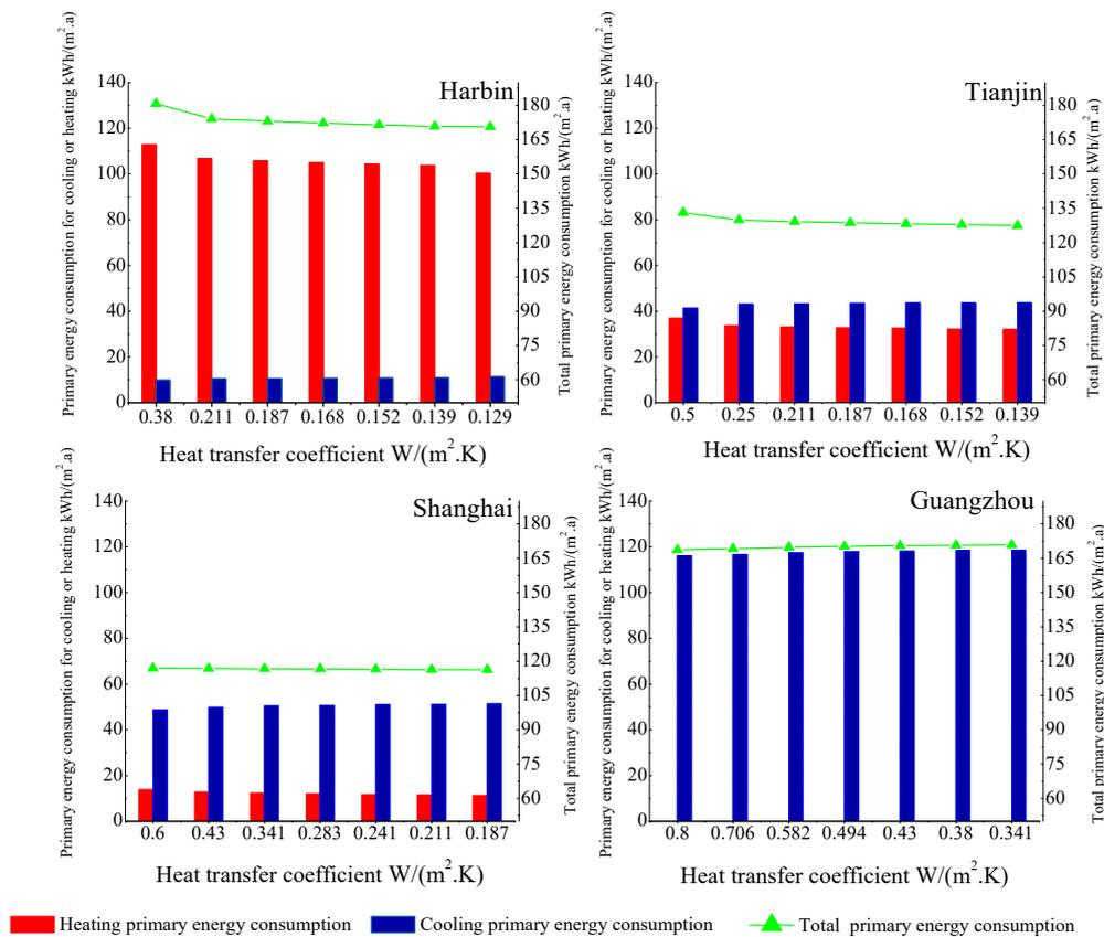
**Figure 5.** Influence of the U-value of exterior wall on primary energy consumption in four cities.
