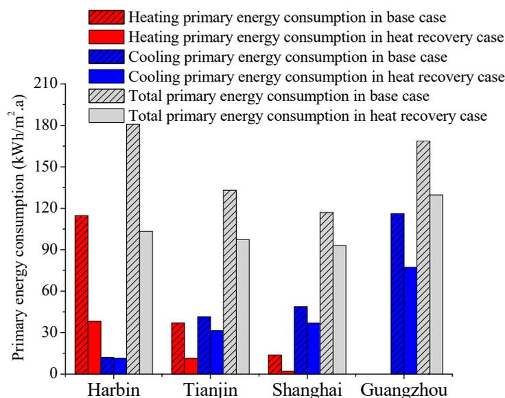
**Figure 16.** Primary energy consumption in air-to-air heat recovery case and base case in four cities.
