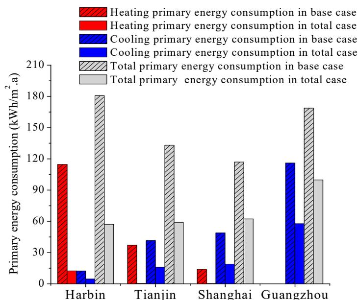
**Figure 19.** Primary energy consumption of integrated design solution and base case in four cities.
