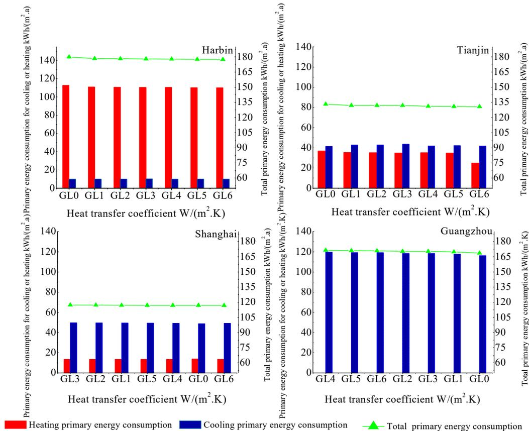
**Figure 7.** The primary energy consumption of different window glass configurations.
