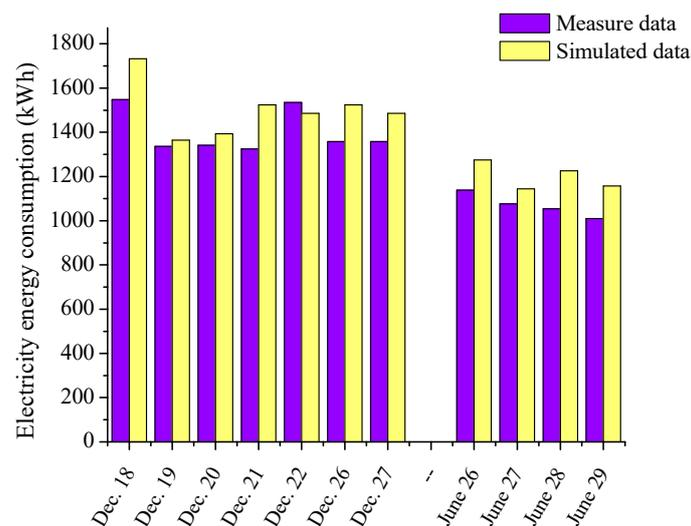
**Figure 3.** The difference between actual electricity energy consumption and simulated data from DesignBuilder (DB).
