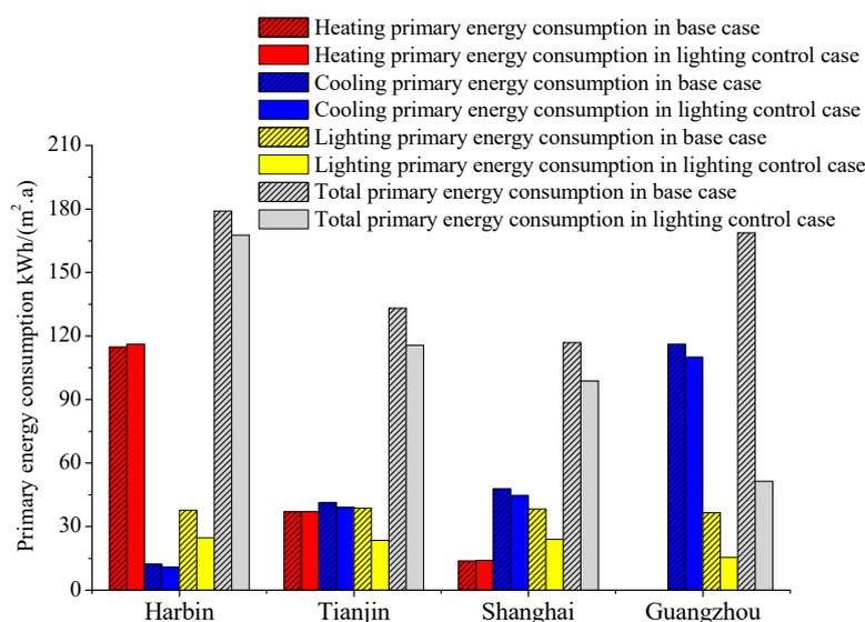
**Figure 15.** Primary energy consumption in lighting control case and base case in four cities.
