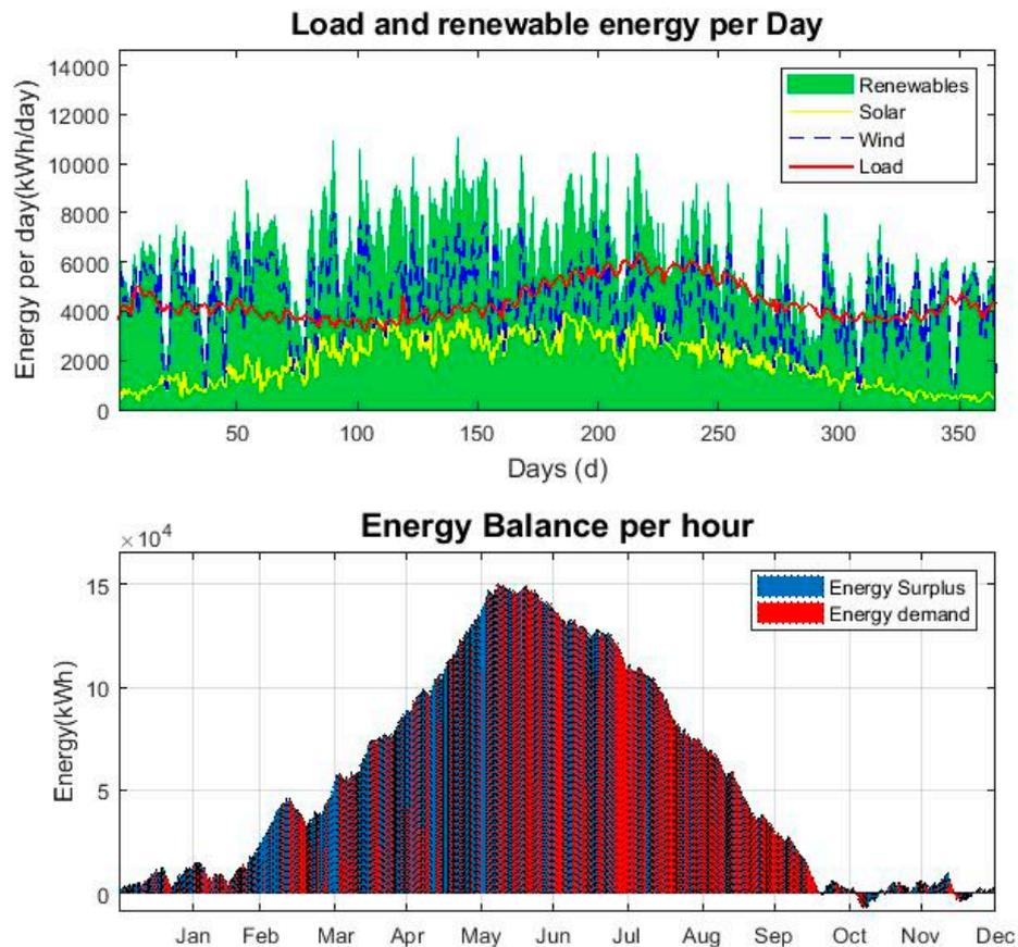
**Figure S4.** Case 1: Scenario 5 instantaneous generation and load variation (top) and energy balance (bottom).
