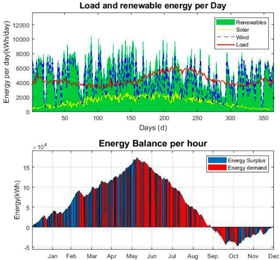
**Figure S5.** Case 1: Scenario 6 instantaneous generation and load variation (top) and energy balance (bottom).
