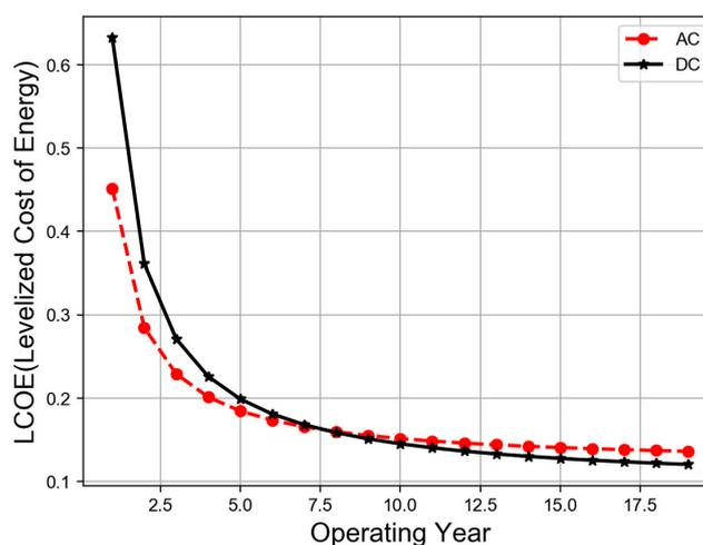
Figure 4. Relationship between LCOE and years of operation in AC and DC distribution networks.
