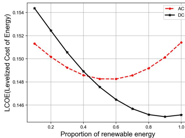
Figure 6. Influence of renewable energy proportion on the LCOE of AC and DC distribution networks.
