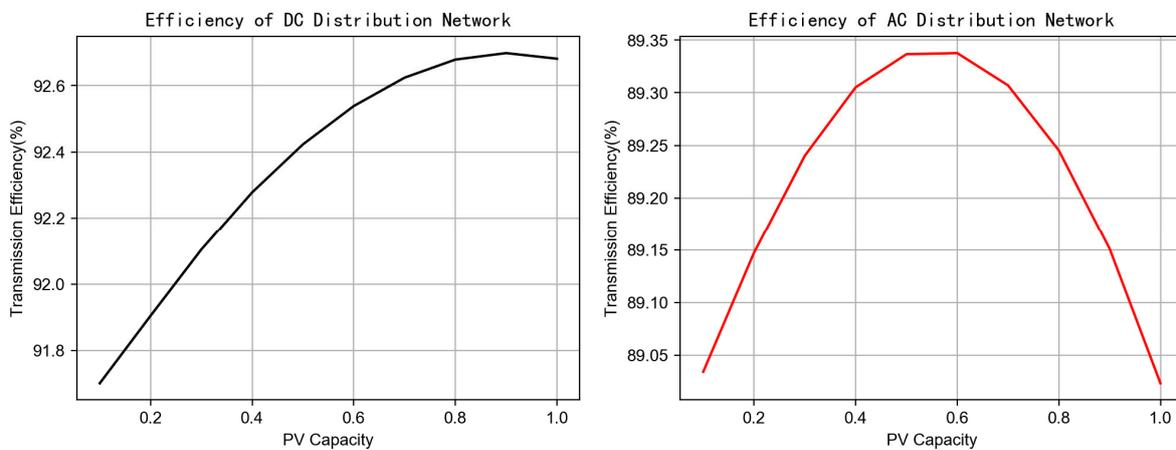
Figure 7. Effect of renewable energy proportion on distribution network efficiency.
