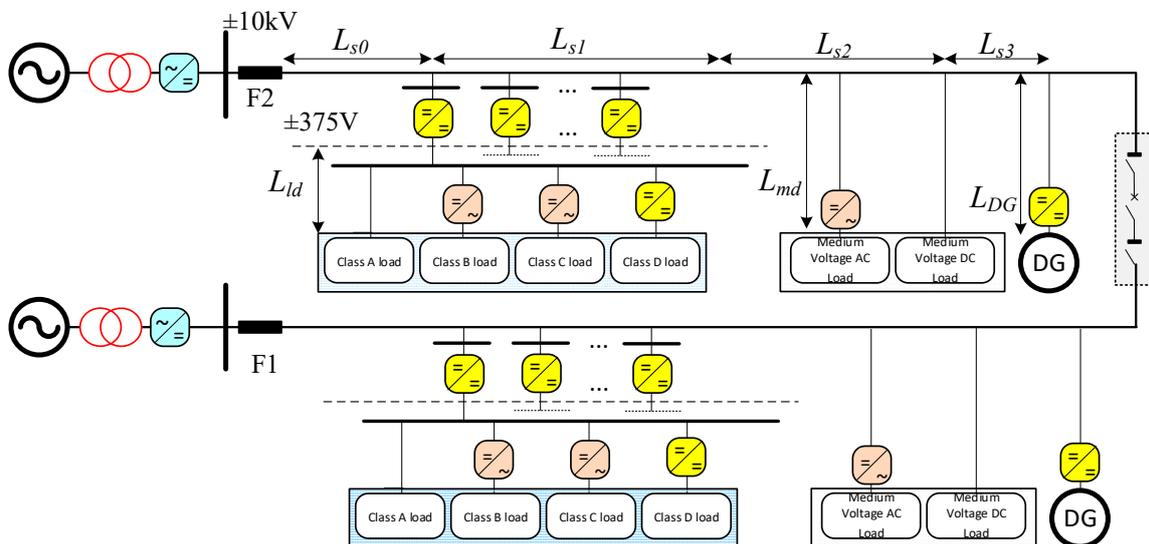
Figure 2. Topology of the DC distribution network.
