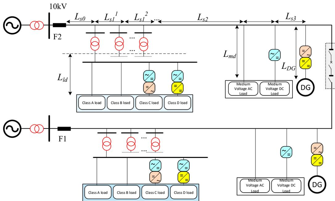
Figure 1. Topology of the AC distribution network.
