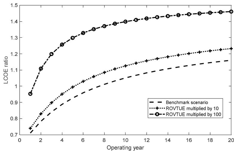
Figure 8. Effect of ROVTUE on LCOE ratio of AC and DC distribution networks.
