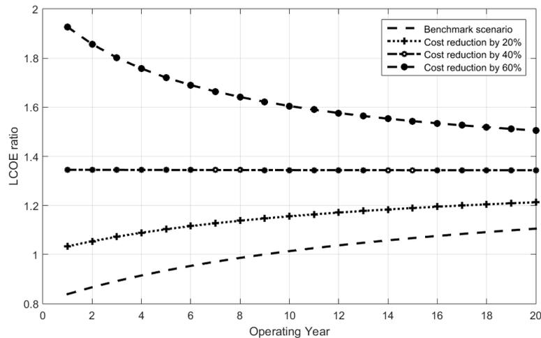
Figure 5. Effect of equipment cost on LCOE ratio of AC and DC distribution networks.
