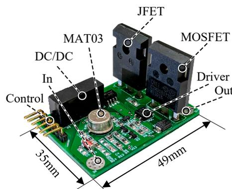
Figure 8. Implemented SSCB-LCL prototype.
