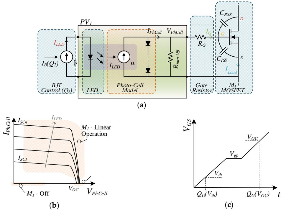
**Figure 2.** (a) Photovoltaic driving circuit block diagram. (b) Ideal current-to-voltage  $PV_1$  characteristic. (c) Gate charge characteristic.
