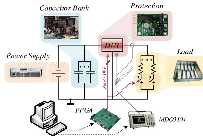
Figure 6. Sketch of the setup for the SSCB-LCL (DUT) validation.
