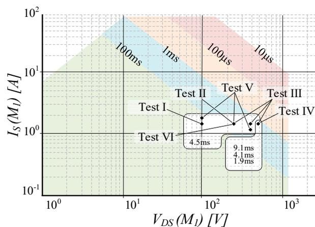
Figure 9. C2M0080120D datasheet Safe Operation Area and theoretical performed test location.
