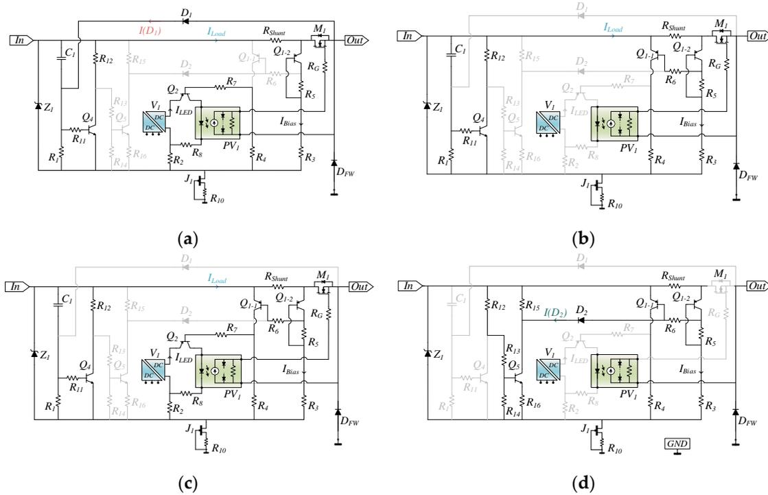
**Figure 4.** Equivalent circuits of each SSCB-LCL state; (a) *On-State*; (b) *Delay state*; (c) *Current Limiting State*; (d) *Off-State*.
