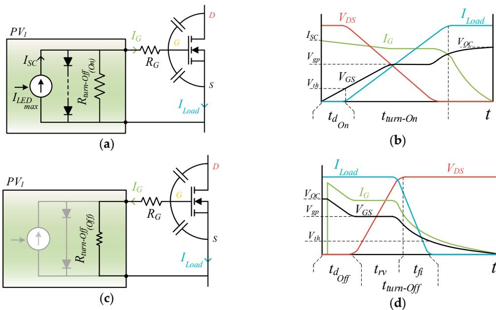
**Figure 3.** (a) Simplified Turn-On circuit; (b) Turn-On transient sketch; (c) simplified Turn-Off circuit; (d) Turn-Off transient sketch.
