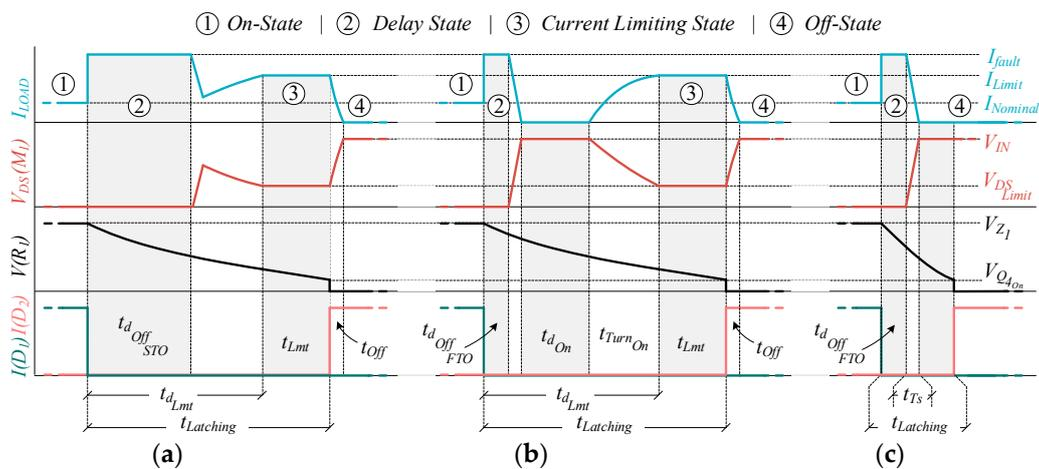
**Figure 5.** Idealized waveforms of each circuit configuration. (a) STO with Current Limitation; (b) FTO with Current Limitation; (c) FTO without Current Limitation (circuit breaker).
