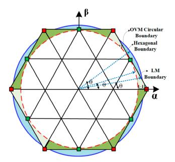
Figure 4. SVD linear modulation (LM) and over modulation (OVM) boundary.
