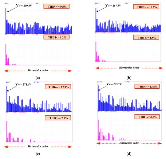
**Figure 18.** Line voltage harmonics spectrum; (a) at  $M_a = 0.7$ , (b) at  $M_a = 0.9$ , (c) at  $M_a = 0.958$ , (d) at  $M_a = 0.997$ .
