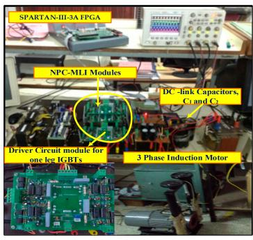
Figure 11. Three-level MLI experimentation with SPARTAN-III-3A XC3SD1800A-FG676 DSP-FPGA.
