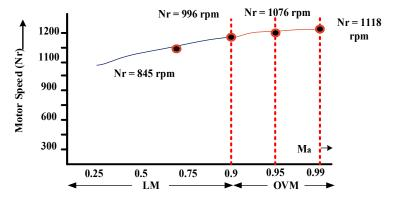
Figure 19. Motor speed response while changing modulation index.
