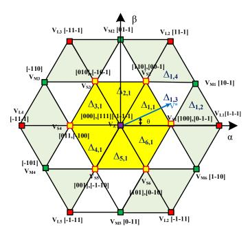
Figure 2. Three-level multilevel inverter (MLI) SVD.
