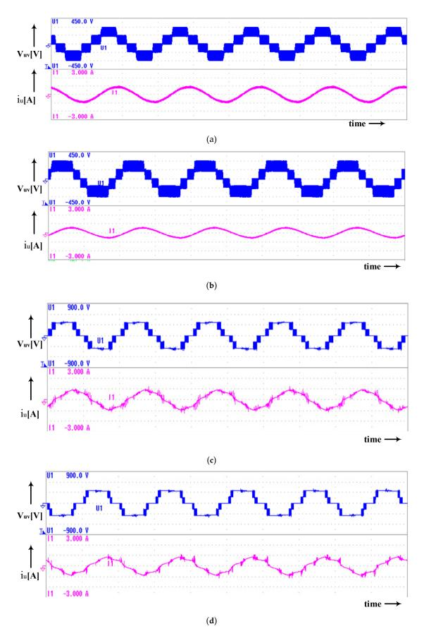
Figure 17. Line voltage  $(V_{uv})$  and Phase current  $(I_u)$  waveform; (a)  $V_{uv}$  for  $M_a=0.7$ , (b)  $V_{uv}$  for  $M_a=0.9$ , (c)  $V_{uv}$  for  $M_a=0.95$ , (d)  $V_{uv}$  for  $M_a=0.99$ .
