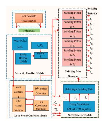
Figure 9. MLI SVM MATLAB-Simulink implementation flow chart.
