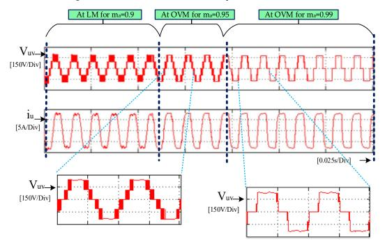
**Figure 10.** Simulation result for modulation range  $(0.9 < M_a \le 0.99)$ .
