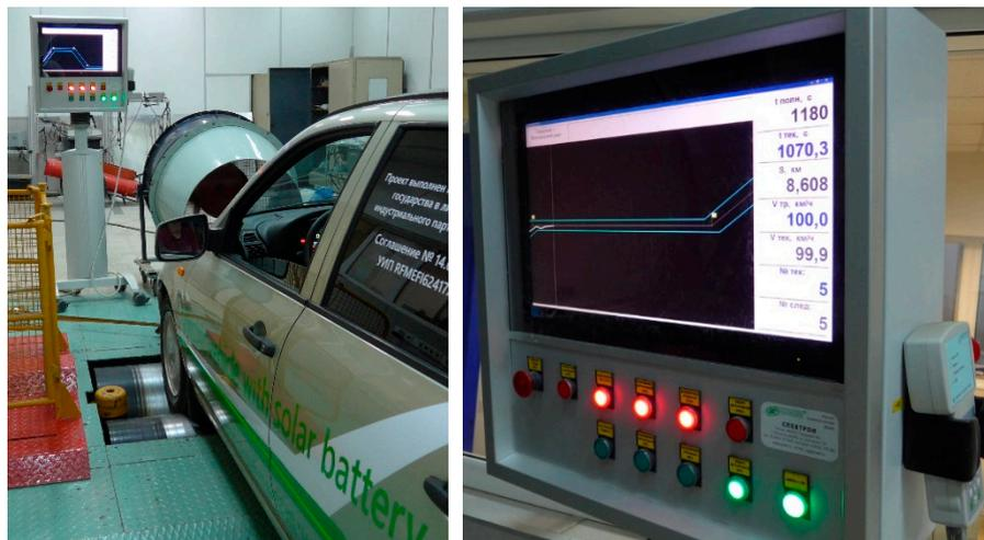
**Figure 10.** Laboratory tests of the developed electric vehicle (on the left: test at the bench with running drums in the driving cycle mode; on the right: speed monitor).
