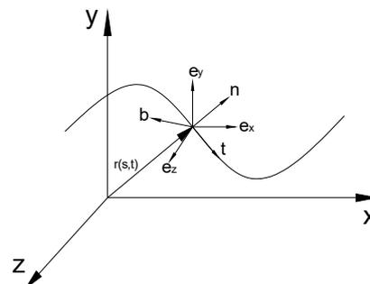
Figure 2. Coordinate system of the beam.
