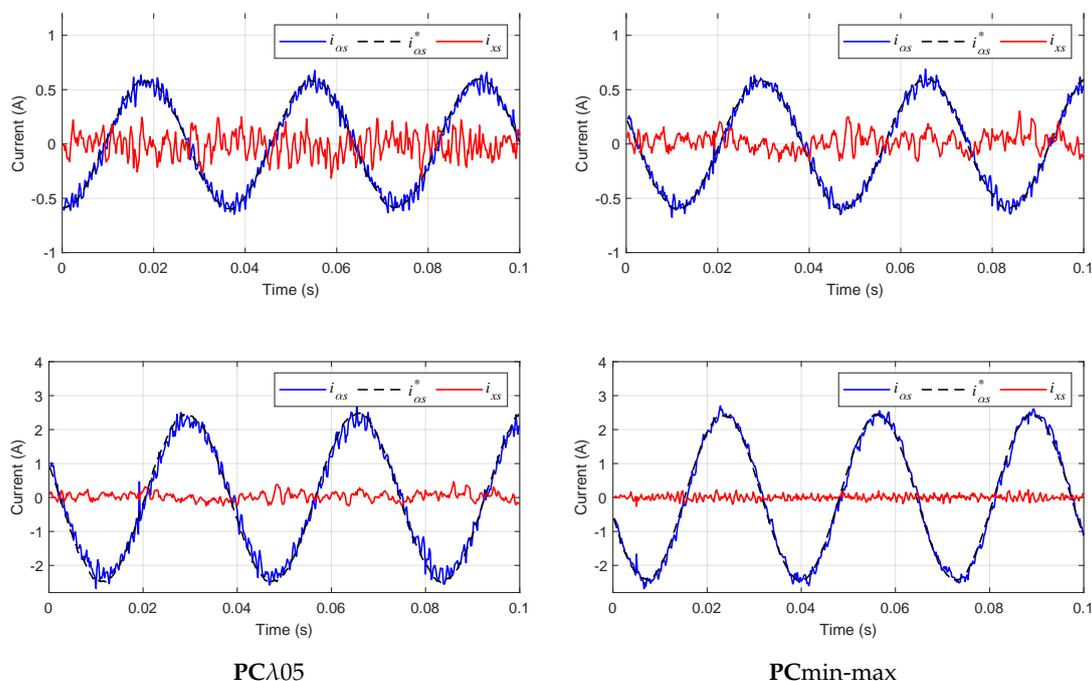
**Figure 2.** Simulation comparison of the proposed controller (right) against a traditional FCSMPC (left) at operating regimes S1 and S2 (top and bottom rows).
