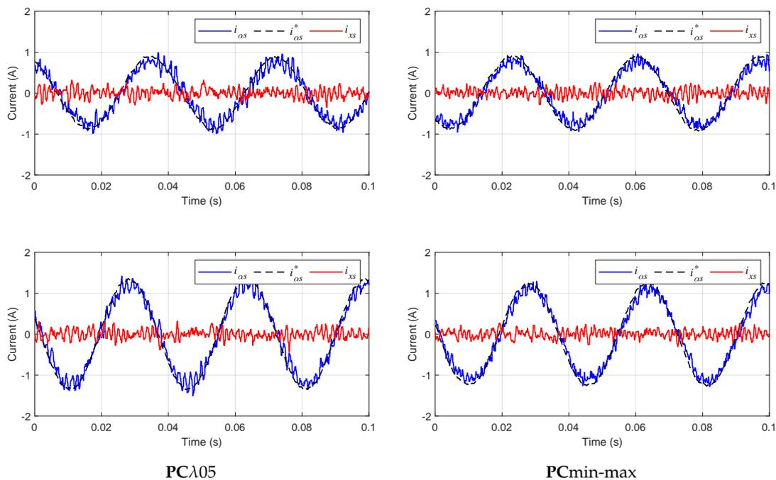
**Figure 4.** Experimental comparison of the proposed controller (right) against a traditional FCSMPC (left) at two operating regimes (top and bottom rows).
