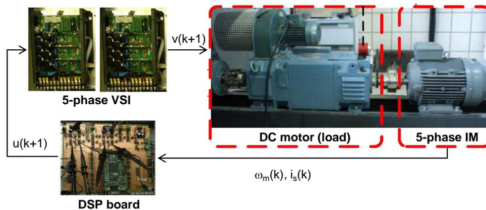
Figure 3. Photographs of the various elements of the experimental setup.
