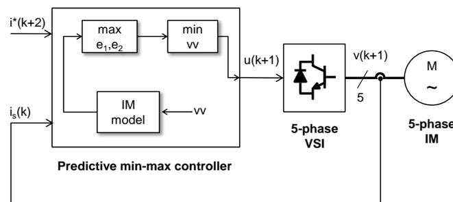
**Figure 1.** Block diagram of min-max Predictive Stator Current Control (PSCC) for a five-phase induction machine (IM) driven by an Voltage Source Inverter (VSI).
