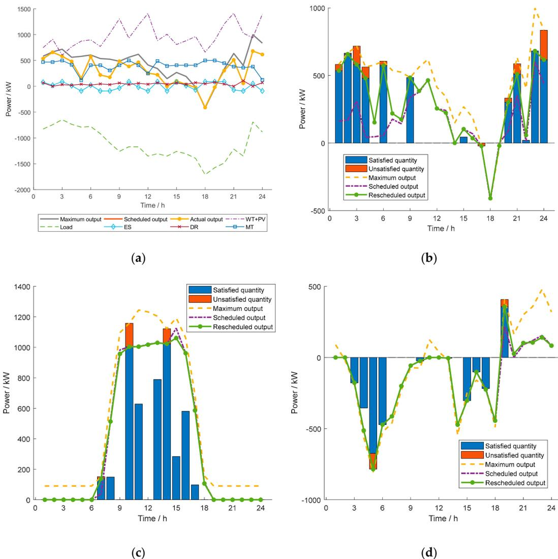
**Figure 9.** Changes in the output and P2P trade quantity of a VPP after rescheduling in the first round of negotiations ( $R = 1$ ): (a) The detailed result of rescheduling VPP<sub>1</sub>; (b) changes in the output and P2P trade quantity of VPP<sub>1</sub> after rescheduling; (c) changes in the output and P2P trade quantity of VPP<sub>6</sub> after rescheduling; (d) changes in the output and P2P trade quantity of VPP<sub>7</sub> after rescheduling.
