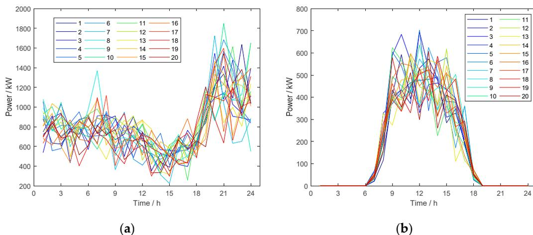
**Figure 5.** Twenty typical scenarios of wind/photovoltaic power in VPP<sub>1</sub>: (a) wind power; (b) photovoltaic power.
