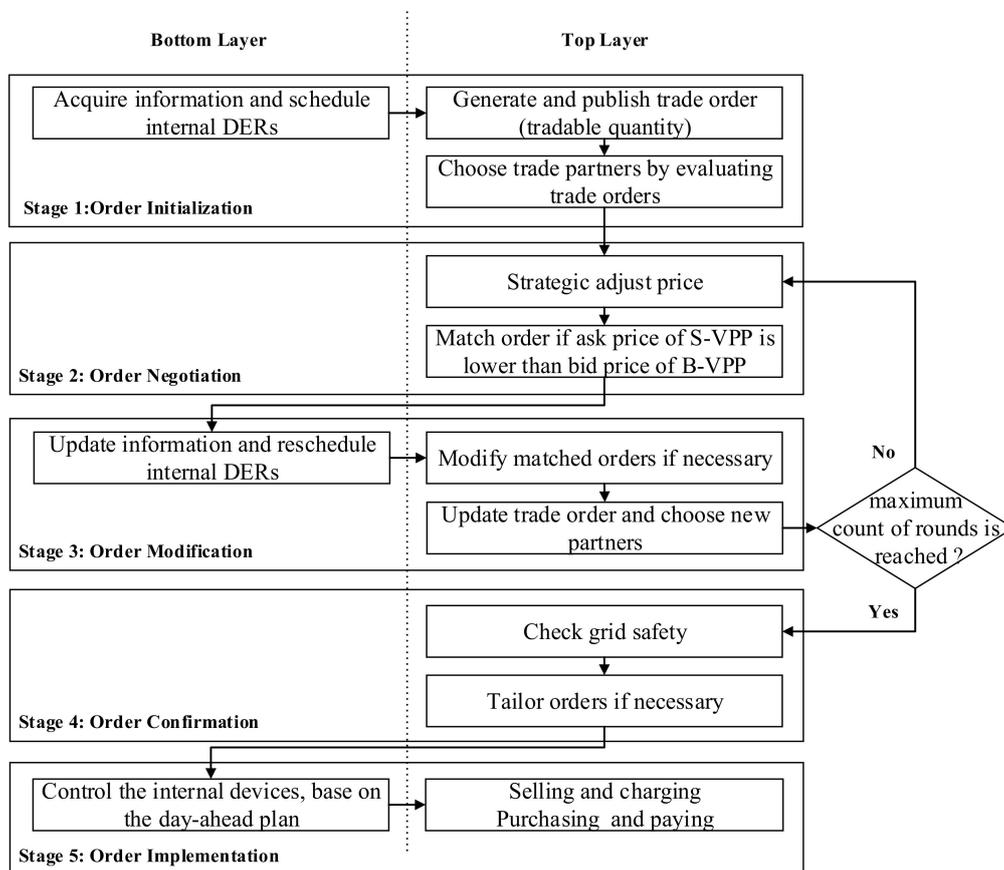
**Figure 2.** Five-stage trade order processing of P2P energy trading. VPP, virtual power plant; DER, distributed energy resource.
