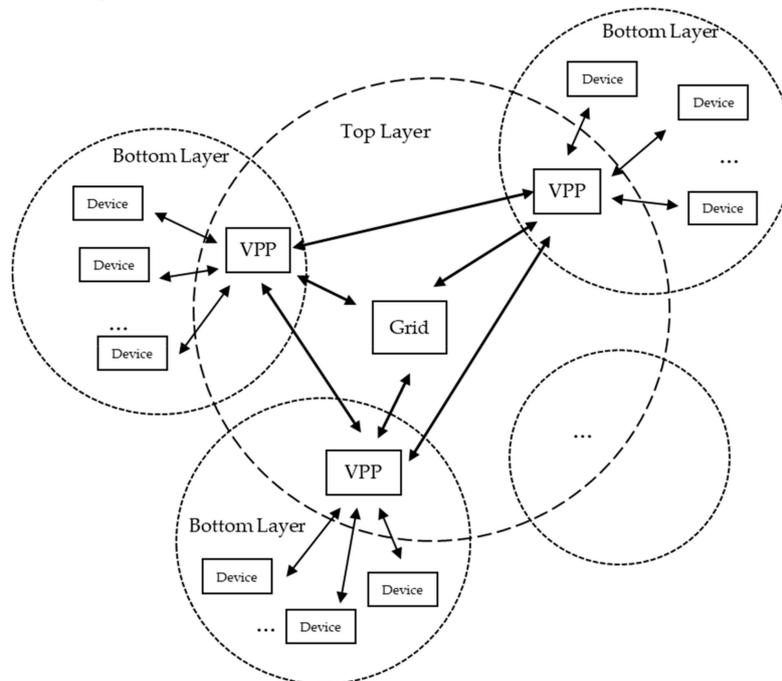
**Figure 1.** Schematic diagram of the peer-to-peer (P2P) energy trading mechanism involving two interactive layers.
