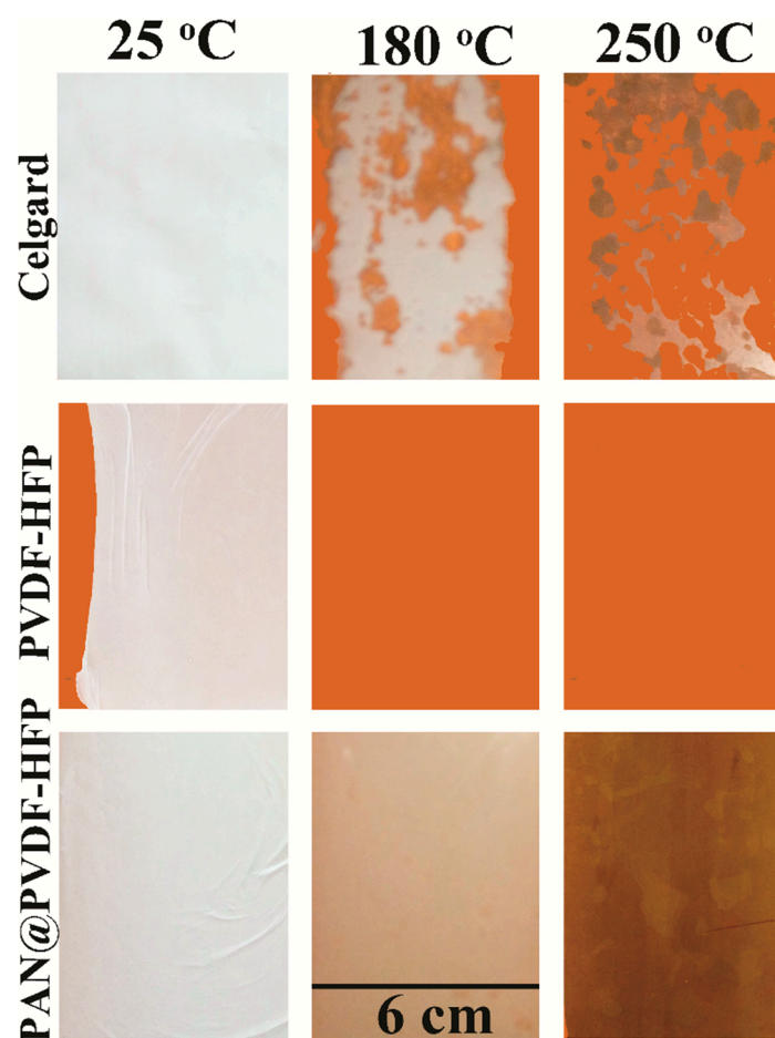
Figure 3. The thermal stability tests of commercial Celgard2400 separator, PVDF-HFP, and PAN@PVDF-HFP fiber network.
