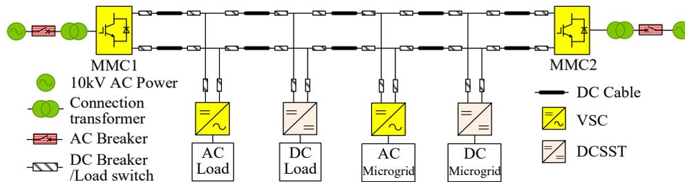
**Figure 1.** Topological structure of the  $\pm 10$  kV VSC-DC distribution system.
