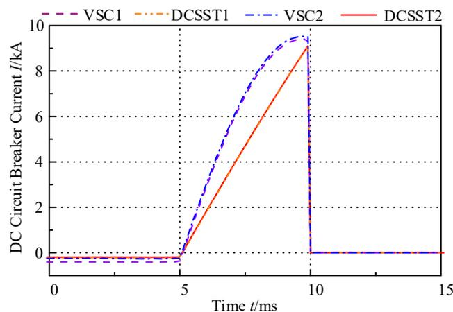
**Figure 17.** The current of the DC circuit breakers in each device under F1 fault.
