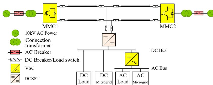
Figure 12. Topological structure of VSC-DC distribution system.
