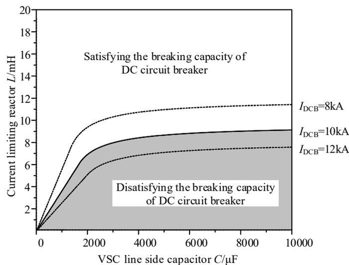
**Figure 8.** Relationship between DC circuit breaker breaking capacity  $I_{DCB}$  and VSC capacitor  $C$ , current limiting reactor  $L_{(VSC)}$ .
