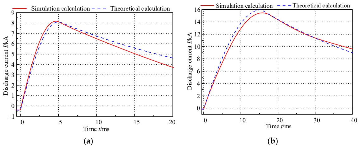
**Figure 14.** The current waveform under F2 fault by theoretical calculation and simulation calculation: (a) VSC1 discharge current when F2 fault occurs in DCSST1 and (b) DCSST1 discharge current when F2 fault occurs in VSC1.
