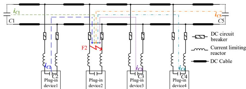
**Figure 11.** When F2 pole-to-pole fault occurs in plug-in device 2, other devices discharge to the fault point.
