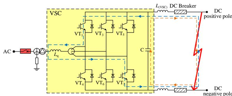
Figure 3. The first stage discharge circuit of VSC fault.
