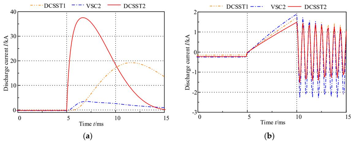
**Figure 16.** The current of DCSST1, VSC2, and DCSST2 under F2 fault in VSC1: (a) without current limiting reactors and (b) with current limiting reactors.
