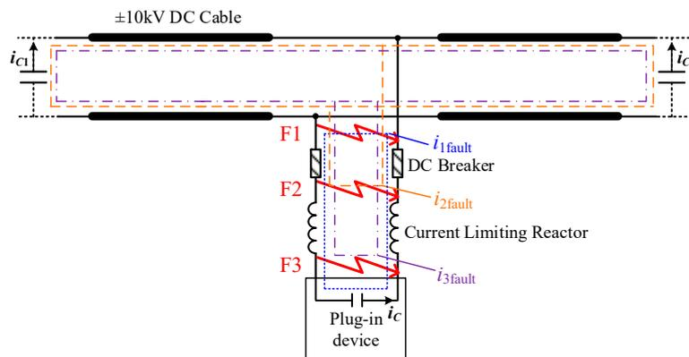
**Figure 2.** The possible pole-to-pole faults at the line side of plug-in devices.
