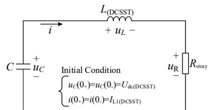
Figure 10. Equivalent circuit of the first stage discharge circuit of DCSST.
