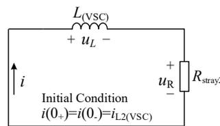
Figure 6. Equivalent circuit of the second stage discharge circuit of VSC.
