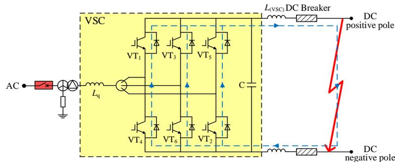
Figure 5. The second stage discharge circuit of VSC fault.
