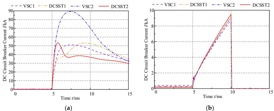
**Figure 15.** The current of the DC circuit breakers in each device under F2 fault: (a) without current limiting reactors and (b) with current limiting reactors.
