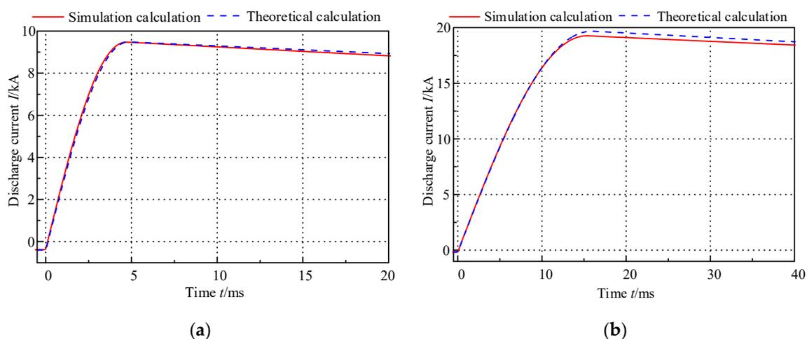
**Figure 13.** The current waveform under F1 fault by theoretical calculation and simulation calculation: (a) VSC1 discharge current and (b) DCSST1 discharge current.
