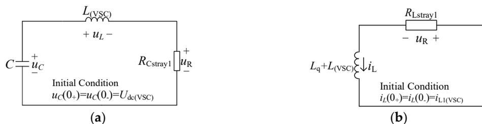
Figure 4. Equivalent circuit of the first stage discharge circuit of VSC: (a) capacitor and inductor discharge equivalent circuit and (b) inductor discharge equivalent circuit.
