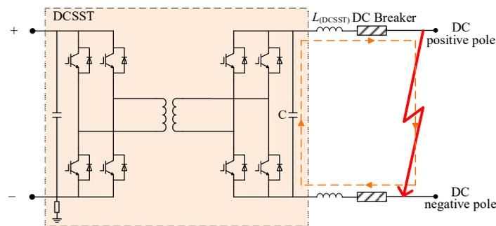
Figure 9. The first stage discharge circuit of DCSST fault.
