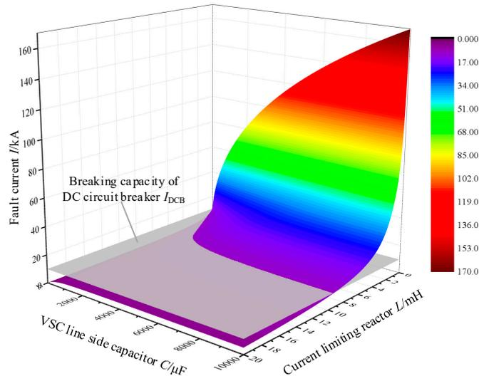
**Figure 7.** Effect of VSC line side capacitor and current limiting reactor ( $C, L_{(VSC)}$ ) on the fault current of DC circuit breaker.
