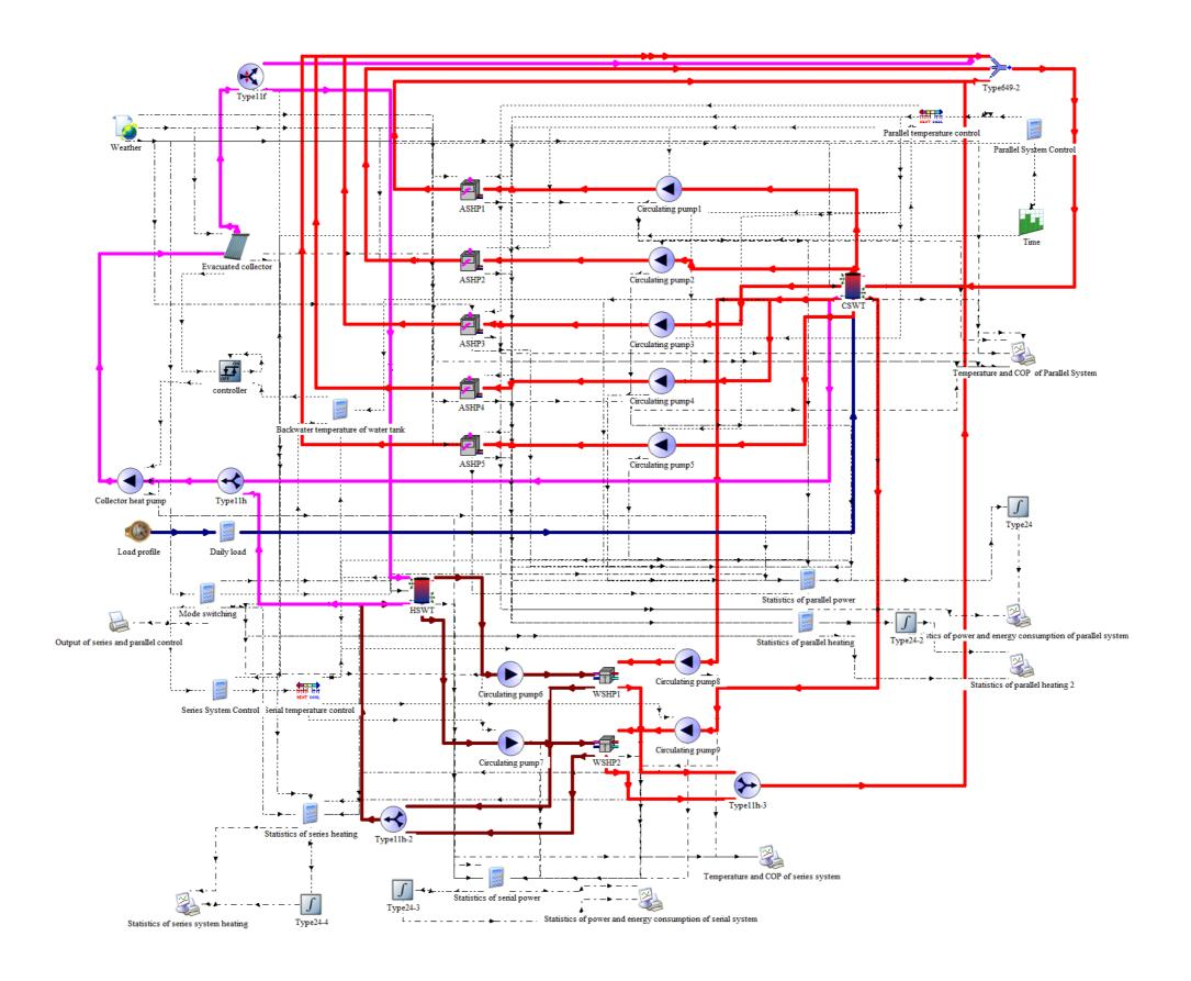
Figure S1. TRNSYS model of the combined SAHP system.
