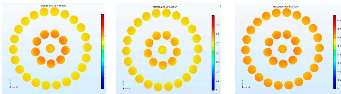
(a) 2 L/m charging flow rate      (b) 3 L/m charging flow rate      (c) 4 L/m charging flow rate
