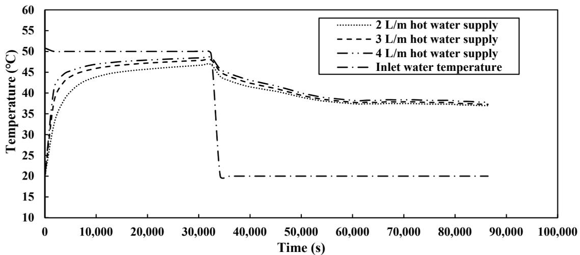
Figure 4. Storage tank inlet and outlet water temperatures.
