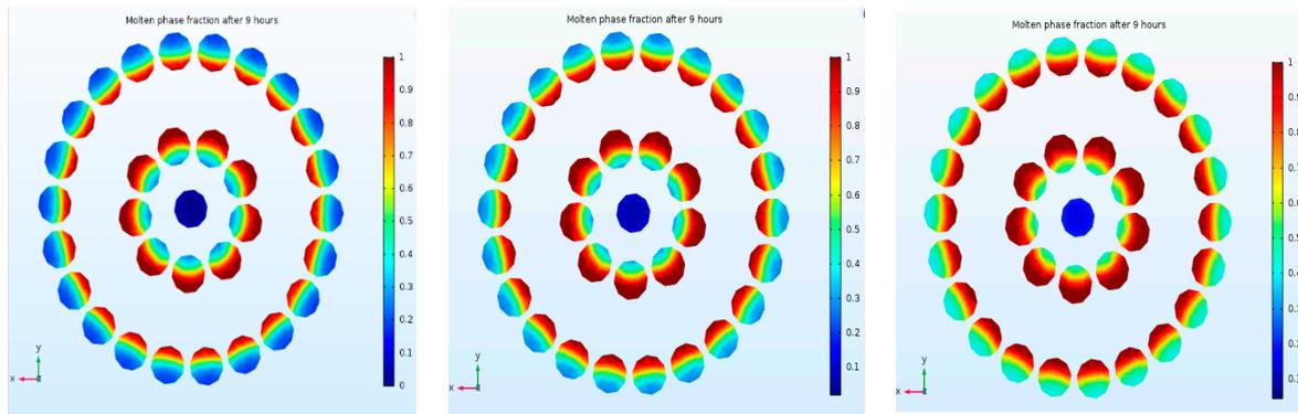
(a) 2 L/m charging flow rate      (b) 3 L/m charging flow rate      (c) 4 L/m charging flow rate
