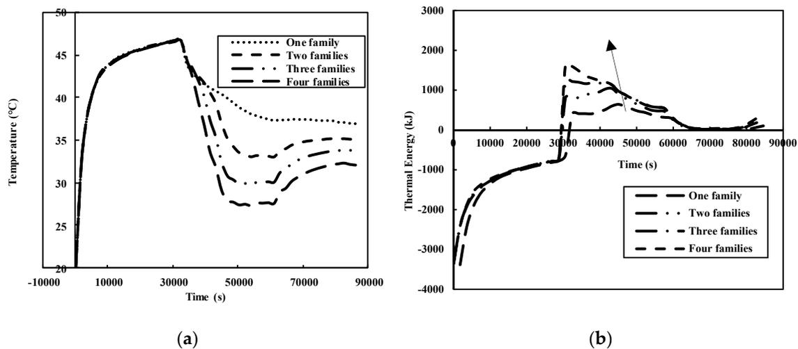
**Figure 9.** Outlet water temperatures and thermal energy over one day of operation. (a) Outlet temperature variation versus number of families; (b) Thermal energy stored and recovered during the day for the demands of one, two, three, and four families.
