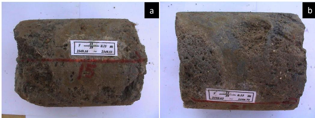
**Figure 7.** Cavern characteristics of the study area (a) Well CT-4, 2343.19~2343.29 m, Cinder-like dolomite (b) Well CT-4, 2344.77~2345.14 m, dissolution caverns in the dolomite rock.
