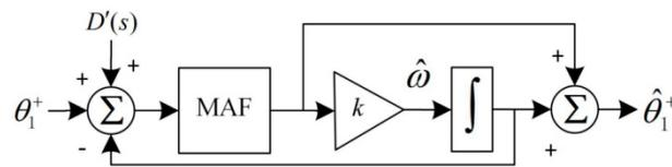
Figure 10. Small-signal model of QT1-PLL.
