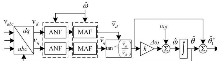
Figure 4. Block scheme of the proposed PLL.
