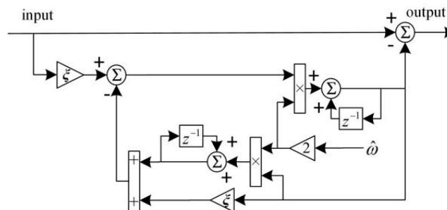
Figure 18. Discrete-time realization of ANF.
