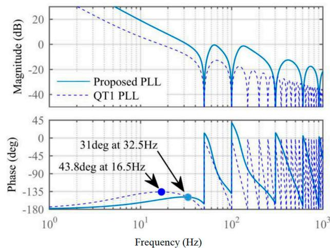
**Figure 16.** Open-loop bode plot of the proposed PLL and QT1-PLL (with dc rejection capability).
