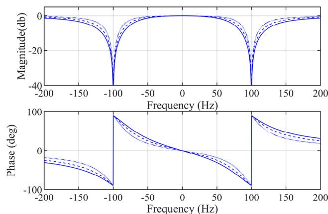
Figure 5. Bode plot of ANF part in filtering stage.  $\zeta = 0.5$  (dotted lines),  $0.7$  (dashed lines),  $0.9$  (solid lines).
