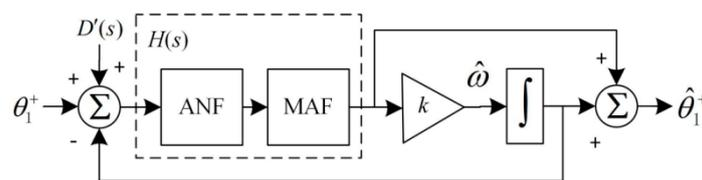
Figure 11. Small-signal model of the proposed PLL.
