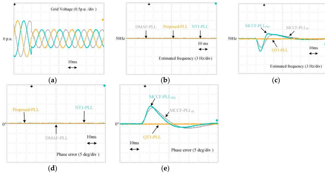
**Figure 24.** Experimental waveforms under a 0.5 p.u. voltage sag: (a) Three-phase voltages; (b,c) Estimated frequency; (d,e) Phase error.
