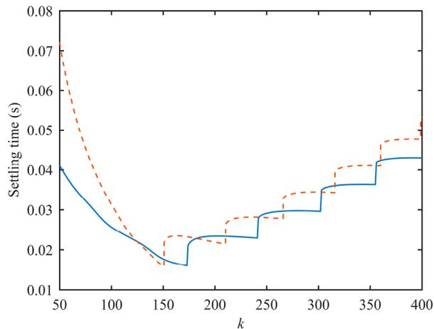
Figure 13. 2% settling time as a function of  $k$ .
