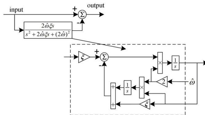
Figure 7. The adaptive structure of ANF.
