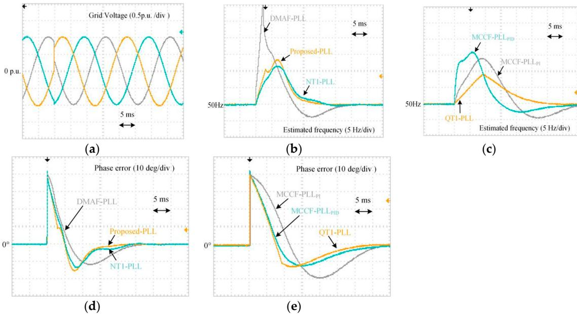
**Figure 21.** Experimental waveforms under a +40° phase jump: (a) Three-phase voltages; (b,c) Estimated frequency; (d,e) Phase error.
