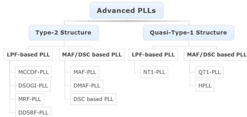
**Figure 2.** A general classification of typical advanced PLLs.
