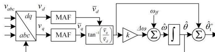
**Figure 3.** Block scheme of QT1-PLL.
