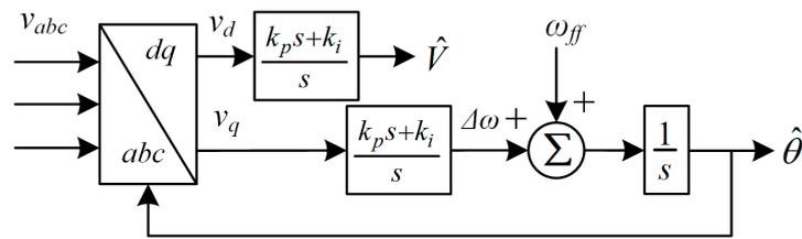
Figure 1. Block schematic of SRF-PLL.
