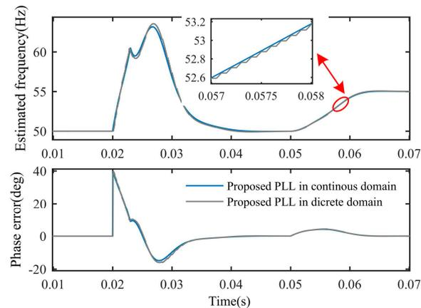
**Figure 19.** The discretization effect of the proposed PLL.
