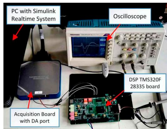
**Figure 20.** Experimental setup.
