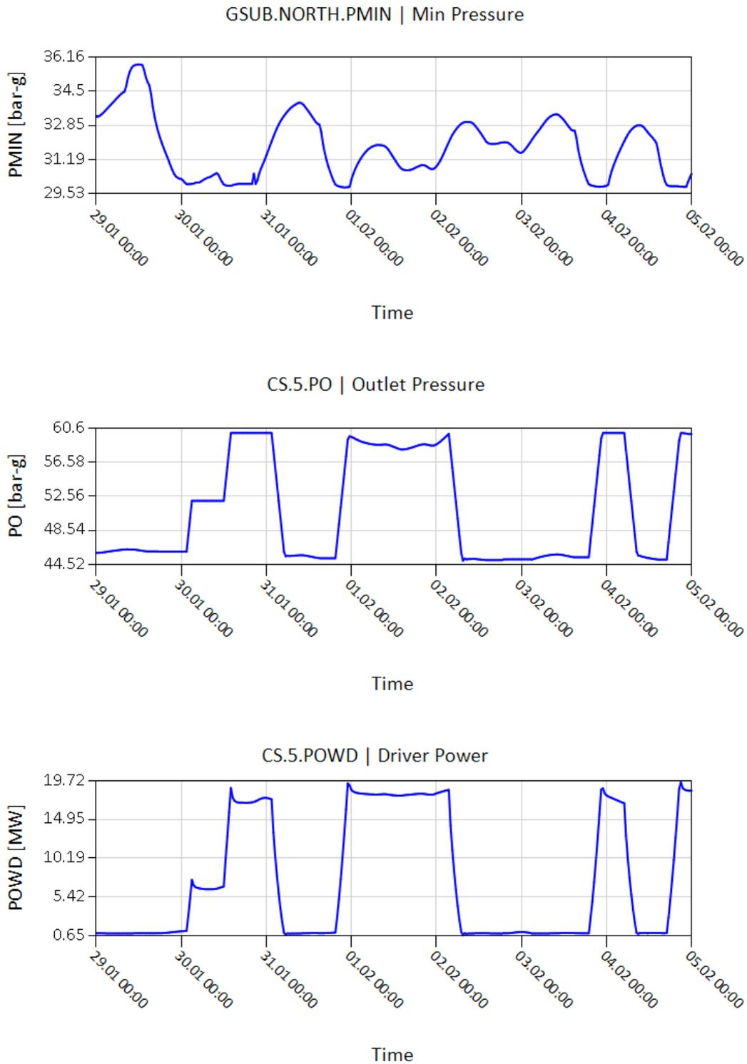
**Figure 11.** Time evolution of minimum pressure in subsystem GSUB.NORTH and outlet pressure and driver power for compressor station CS.5 for DA simulation for Q1 and for a 20% wind and solar penetration.
