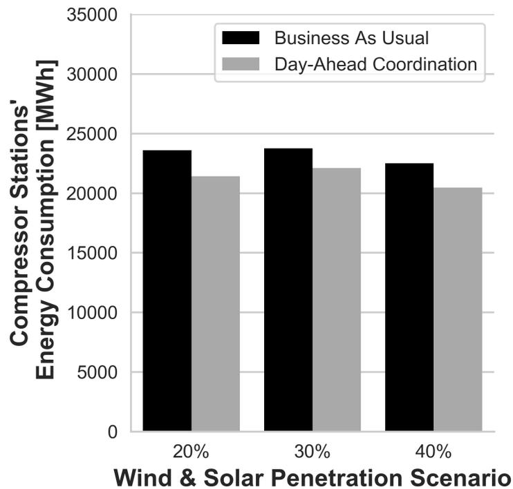
**Figure 9.** Total energy consumption of gas compressor stations in the Business As Usual and DA Coordination case. Aggregated results for four weeks (one per quarter) with highest system-wide natural gas offtake ramps.
