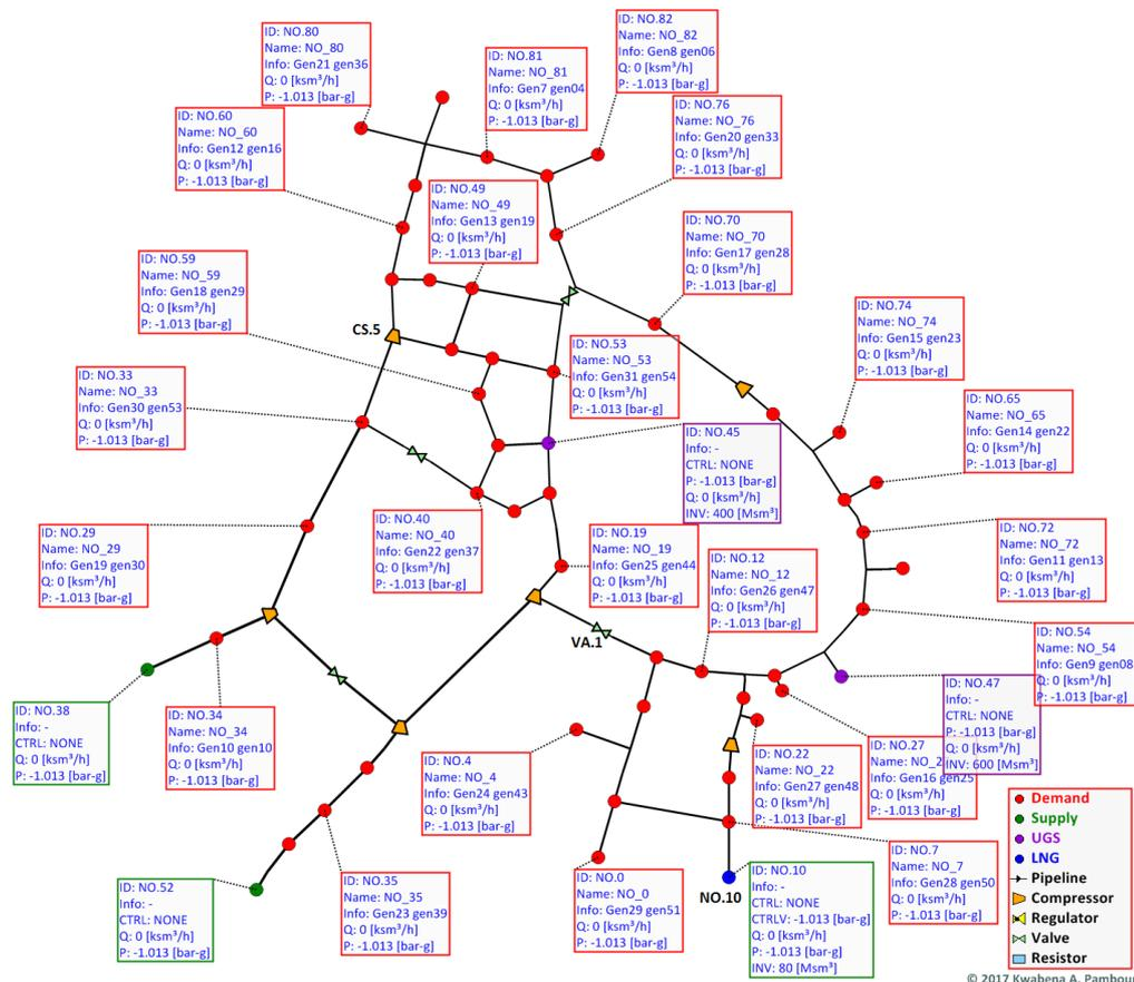
**Figure 2.** Topology of the GNET90 gas network. Labels with a red frame are pointing to gas fired power plant (GFPP), labels with a green frame indicate supply nodes, and those with a purple frame underground gas storage (UGS) facilities.
