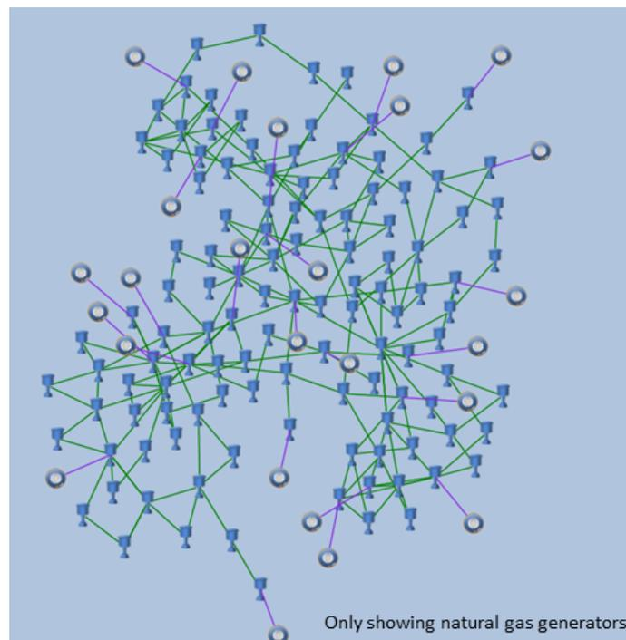
**Figure 1.** Topology of the IEEE 118-Bus power system network.
