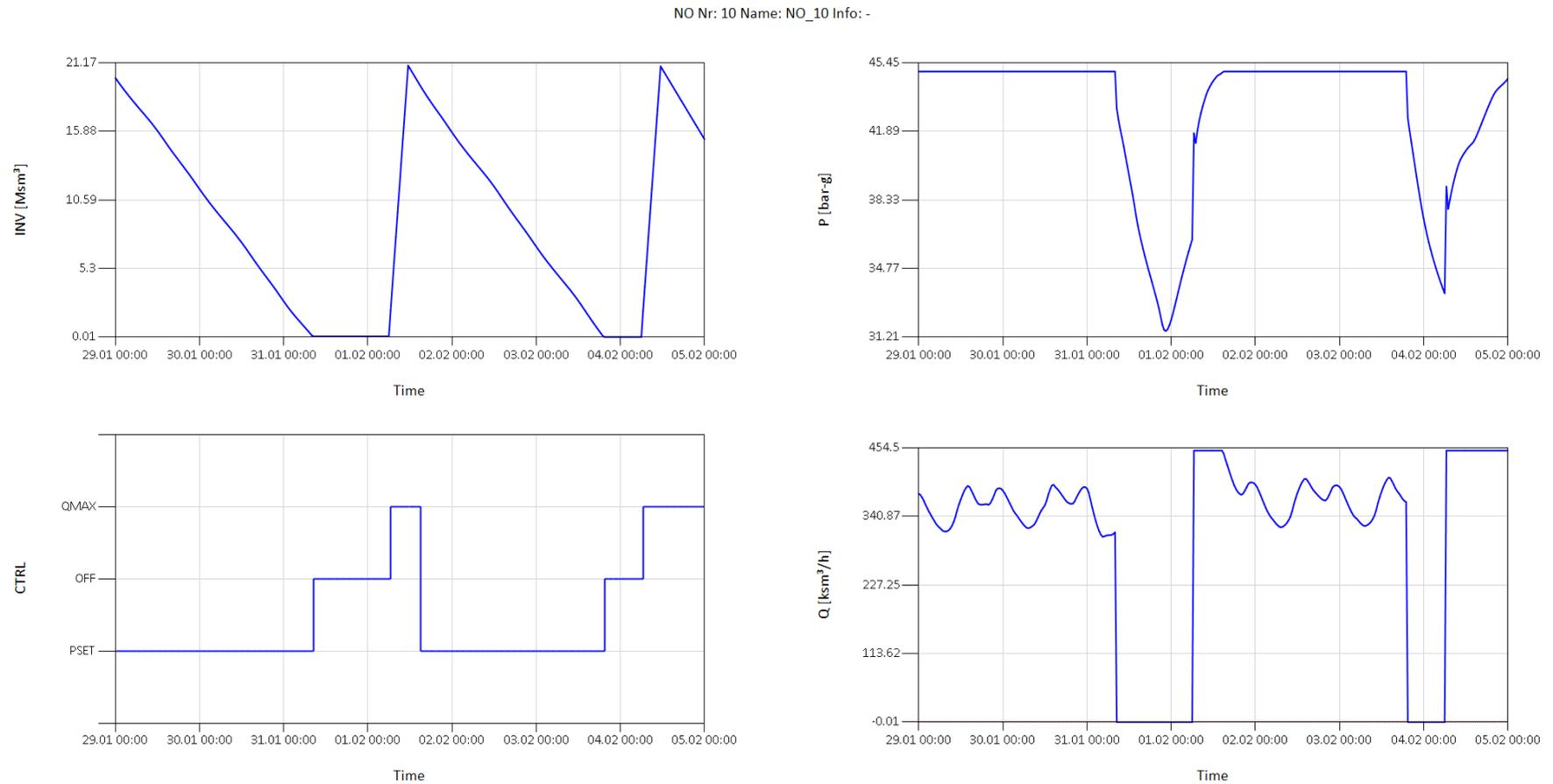
**Figure 12.** Time evolution of working gas inventory (NO.10.INV), station control (NO.10.CTRL), pressure (NO.10.P) and gas supply (NO.10.Q) at liquefied natural gas (LNG) Terminal NO.10 for DA simulation for Q1 and for a 20% wind and solar penetration.
