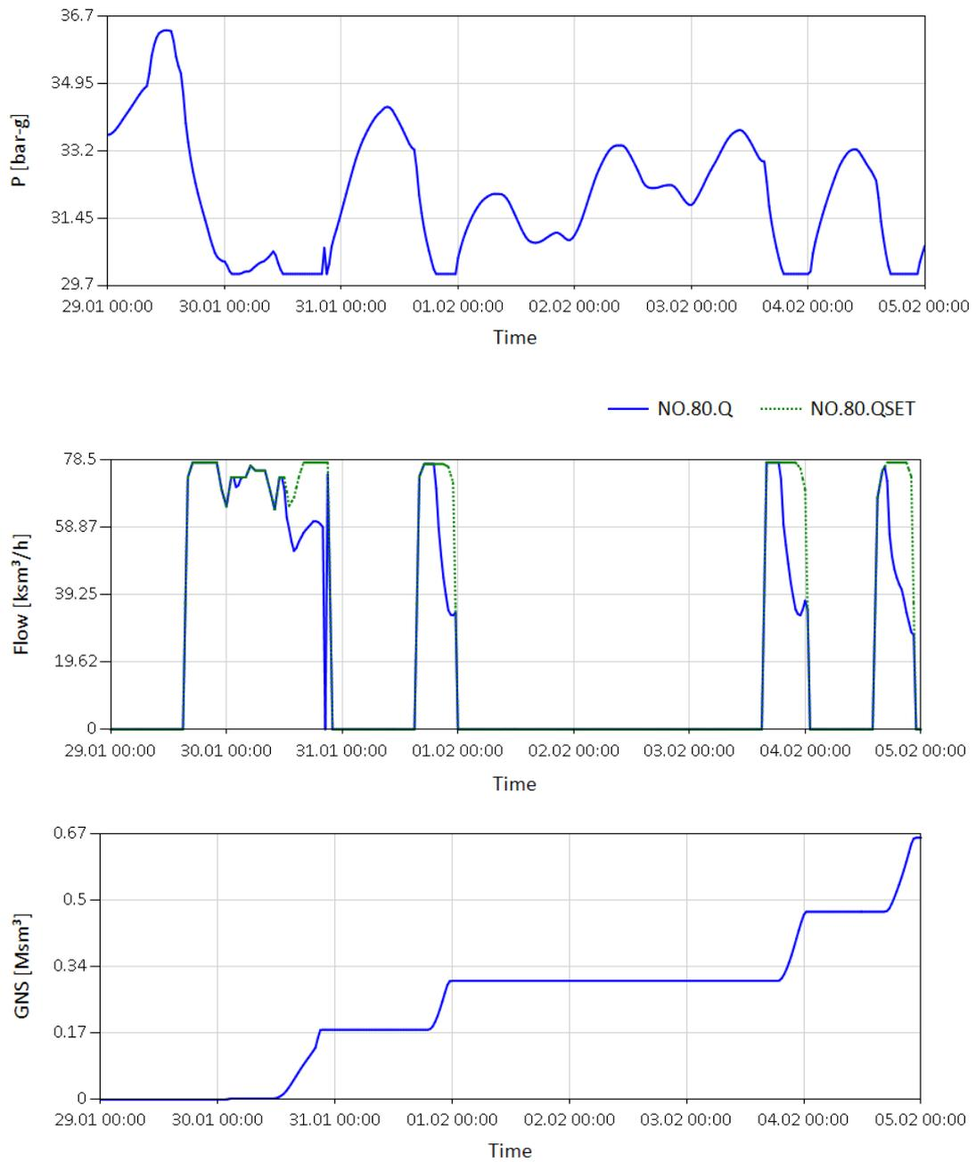
**Figure 10.** Time evolution of pressure, scheduled offtake, actual offtake, and cumulative gas not supplied for fuel offtake node NO.80 of gas generator gen36 for DA simulation for Q1 and for a 20% wind and solar penetration.
