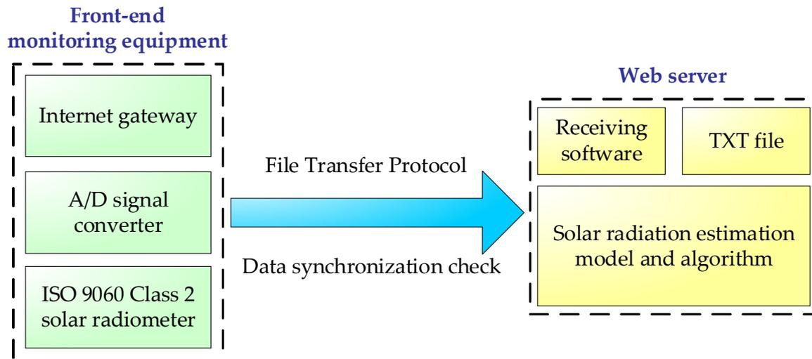
Figure 2. Horizontal solar radiation monitoring system architecture.
