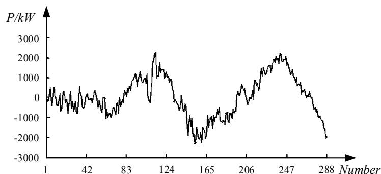
**Figure 4.** Ideal power value of the hybrid energy storage systems (HESS),  $P_{HESS}^*$ .
