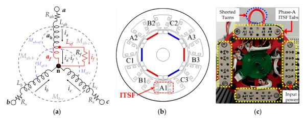
**Figure 1.** IPMSM with ITSF in Phase-A. (a) Equivalent circuit of three-phase IPMSM with ITSF in Phase-A; (b) FEM model of a 400-watt IPMSM with shorted turns in the A1 tooth of phase-A; (c) 400-watt IPMSM with ITSF tabs.
