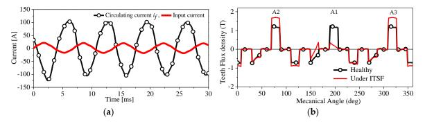
**Figure 2.** (**a**) Stator input current and the circulating/fault current under ITSF; (**b**) Magnetic flux density in teeth of Phase-A under healthy and ITSF conditions.
