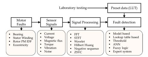
**Figure 4.** Block diagram of the various faults in the motor, signal used as the sensor, signal processing techniques, and the fault detection methods.
