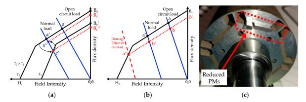
**Figure 3.** Operating point and demagnetization curve of PM due to: (**a**) External demagnetizing MMF; (**b**) Operation at high temperature (NdFeb or SmCo magnets); (**c**) IPMSM rotor with replaceable reduced size PMs.
