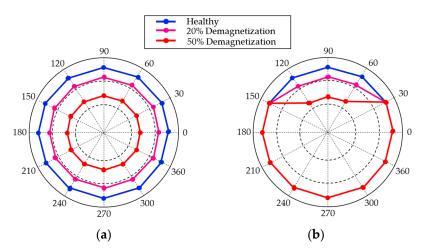
Figure 9. Magnetic field component. (a) Uniform demagnetization; (b) Partial demagnetization.
