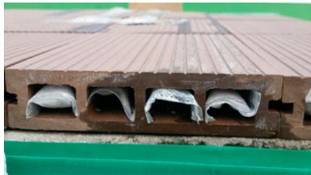
**Figure 2.** Packed PCM placed within the hollows of the wood-plastic composite (WPC) plate.
