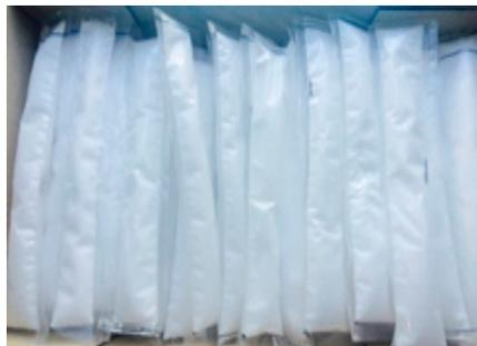
**Figure 1.** Packed phase-change material (PCM) in nylon plastic bags.
