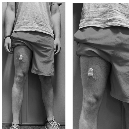
Figure 2. activPAL3 fitting and placement on the participants' midline of the anterior aspect of their right thigh, using a nitrile sleeve and waterproof Tegaderm.
