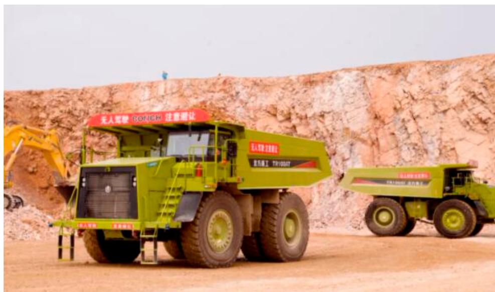
**Figure 3.** (Source from the Internet: [https://www.xianjichina.com/special/detail\\_482389.html](https://www.xianjichina.com/special/detail_482389.html), accessed on 26 March 2022) China Conch Group's driverless mining trucks [64].
