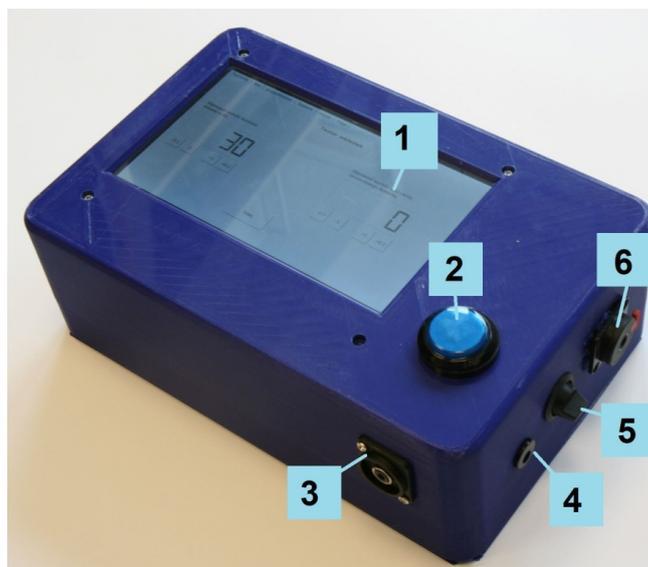
**Figure 3.** The implemented tester: Diagonal view (1. LCD with a touch panel, 2. response button, 3. headphone connector, 4. charging connector, 5. on/off switch, 6. 6.5 mm jack connector for an additional external response button added for testing purposes).
