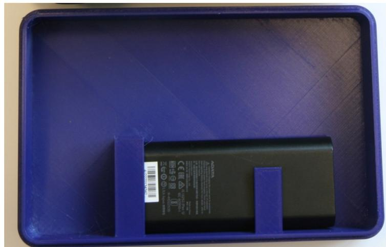
**Figure 5.** The implemented tester: Lower housing cover with the tester's supply battery fitted.
