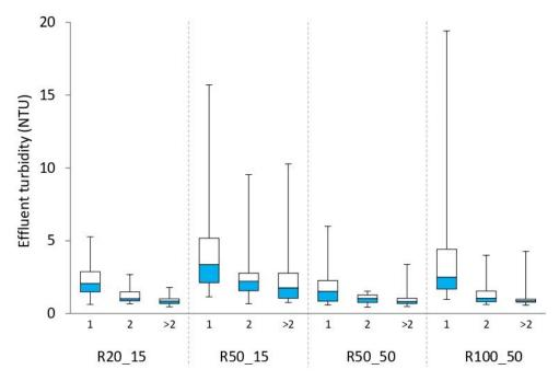
**Figure 6.** Box plots of the permeate turbidity datasets measured at the steady state, excluding the first transient period equal to twice the SRT. For each test, three classes were distinguished according to the number of days since the last mesh cleaning. Run Rx\_y corresponds to "x" mesh pore size  $(\mu m)$  and "y" SRT (d).
