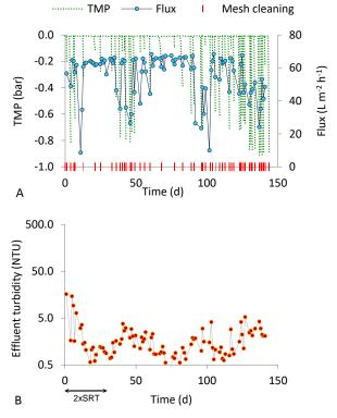
**Figure 3.** Results obtained in run R20 $_1$ 5 (20  $\mu$ m pore size, 15 d SRT). (**A**) Flux, TMP and mesh cleaning; (**B**) effluent turbidity.
