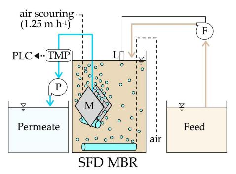
**Figure 1.** Plant scheme of the Self-Forming Dynamic Membrane BioReactor (SFD MBR). P, permeate pump; TMP, manometer with transmembrane pressure transducer connected to a PLC; M, filtration module; F, feed pump; L, level control connected to F.
