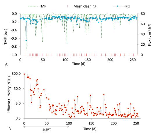
**Figure 5.** Results obtained in run R100\_50 (100  $\mu$ m pore size, 50 d SRT). (**A**) Flux, TMP and mesh cleaning; (**B**) effluent turbidity.
