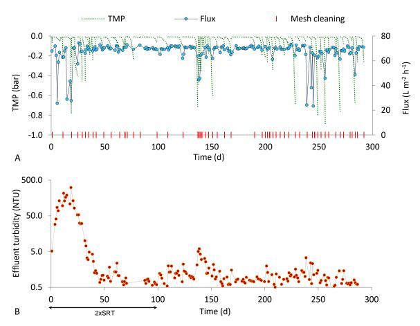
**Figure 4.** Results obtained in run R50\_50 (50  $\mu$ m pore size, 50 d SRT). (**A**) Flux, TMP and mesh cleaning; (**B**) effluent turbidity.
