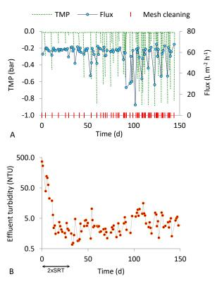
**Figure 2.** Results obtained in run R50\_15 (50  $\mu$ m pore size, 15 d SRT). (**A**) Flux, TMP and mesh cleaning; (**B**) effluent turbidity.
