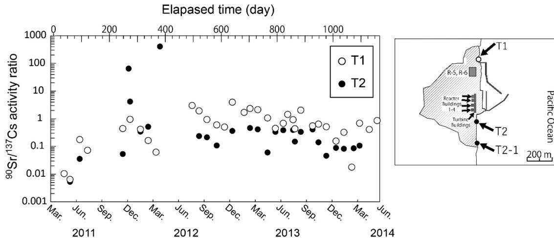
**Figure 1.** Temporal variations of strontium-90/cesium-137 ( $^{90}\text{Sr}/^{137}\text{Cs}$ ) activity ratio in seawater from monitoring sites T1 and T2 (T2-1) in the Fukushima Daiichi Nuclear Power Plant (FDNPP) site [6]. T1 and T2 (T2-1) sites are located north and south of the discharge channel of the FDNPP, respectively.
