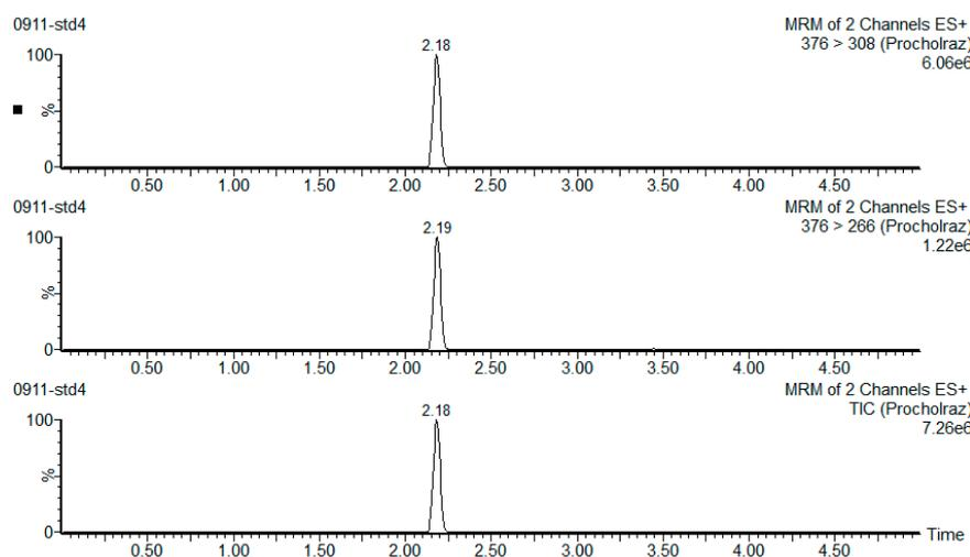
**Figure 1.** An example of an extracted multiple reaction monitoring mode (MRM) chromatogram of a garlic sprout sample, indicating the presence of prochloraz.
