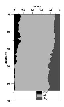
Figure 2. Changes of sediment grain size with depth.
