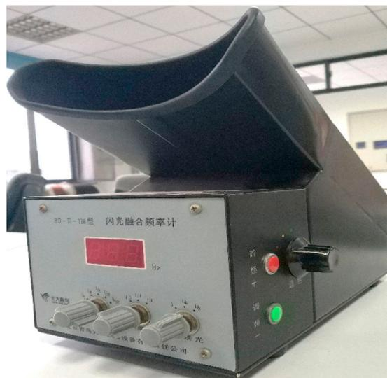
Figure 4. EP403 highlight scintillometer.
