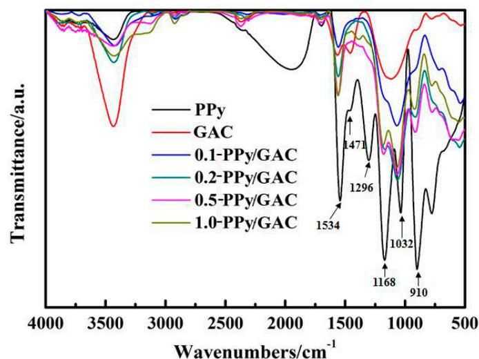
Figure 2. FT-IR spectra of the prepared adsorbents.
