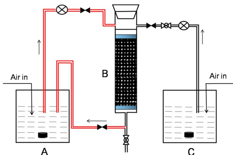
**Figure 1.** Schematic diagram of the laboratory column experiments showing the culture vessel (A); reactor with different adsorbents (B); and MTBE-containing (Methyl *tert*-butyl ether) solution vessel (C). The red line represents recirculation through the feeding vessel (closed mode operation), and the black line represents circulation through the column only (open mode operation). Both the vessel and reactor were maintained at 30 °C.
