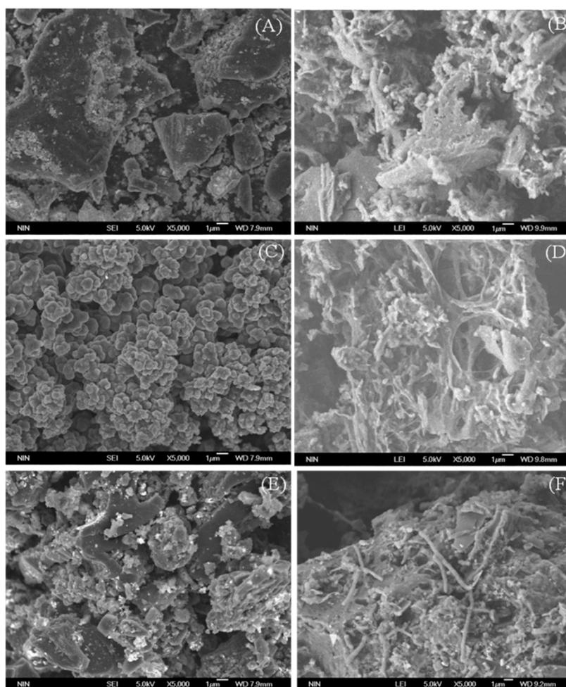
**Figure 7.** SEM graphs of different adsorbents before (A,C,E) and after (B,D,F) the bioreactor operation. (A,B) are of GAC adsorbents; (C,D) are of PPy adsorbents; and (E,F) are of 0.2-PPy/GAC adsorbents.
