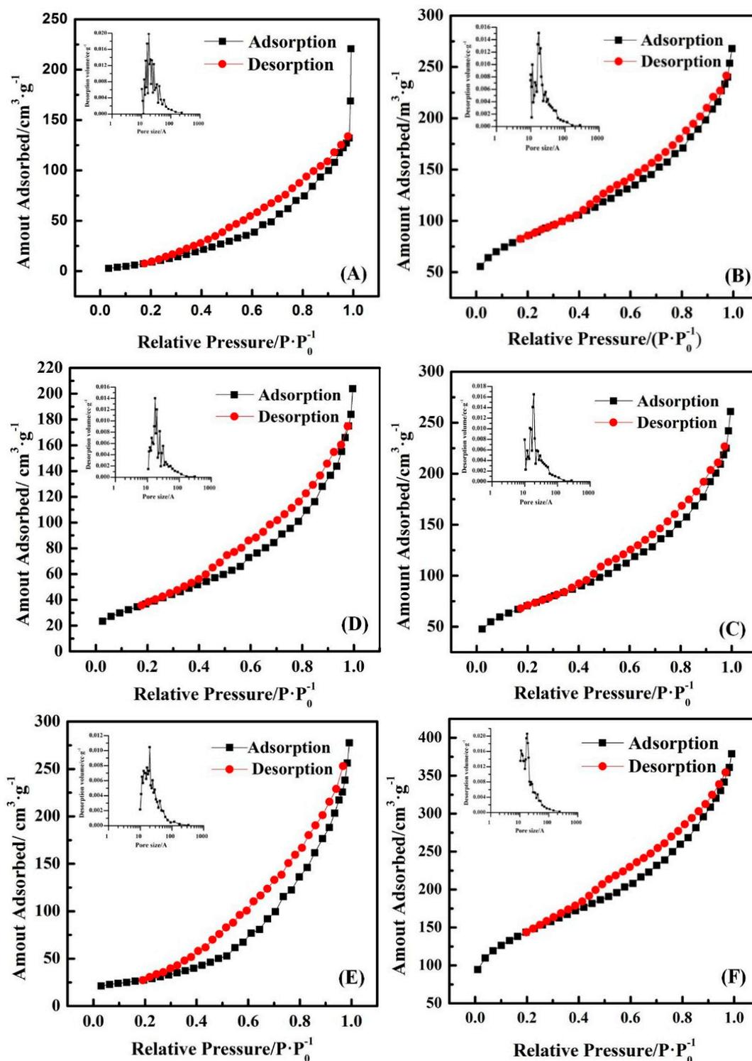
**Figure 3.** Adsorption-desorption isotherms of  $N_2$  of the adsorbents. PPy (A); 0.1-PPy/GAC (B); 0.2-PPy/GAC (C); 0.5-PPy/GAC (D); 1-PPy/GAC (E) and GAC (F).
