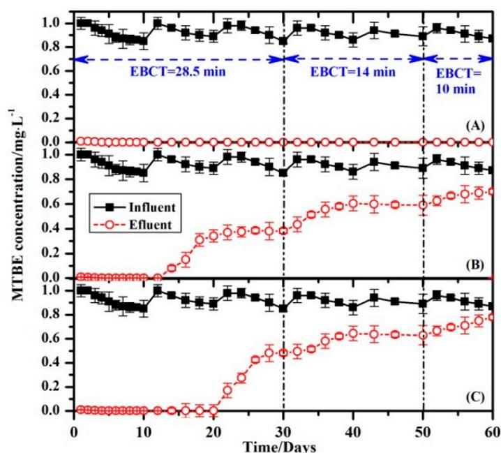
**Figure 5.** Biological filtration of MTBE through laboratory columns with 0.2-PPy/GAC (A); PPy (B); and GAC (C) as adsorbents. The error bars represent the standard deviations from replicate measurements.
