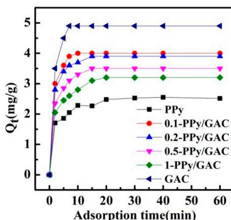
Figure 4. Adsorption equilibrium curves of MTBE on different adsorbents.
