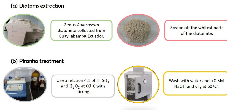
Figure 7. Diatom extraction (a) and piranha treatment (b).
