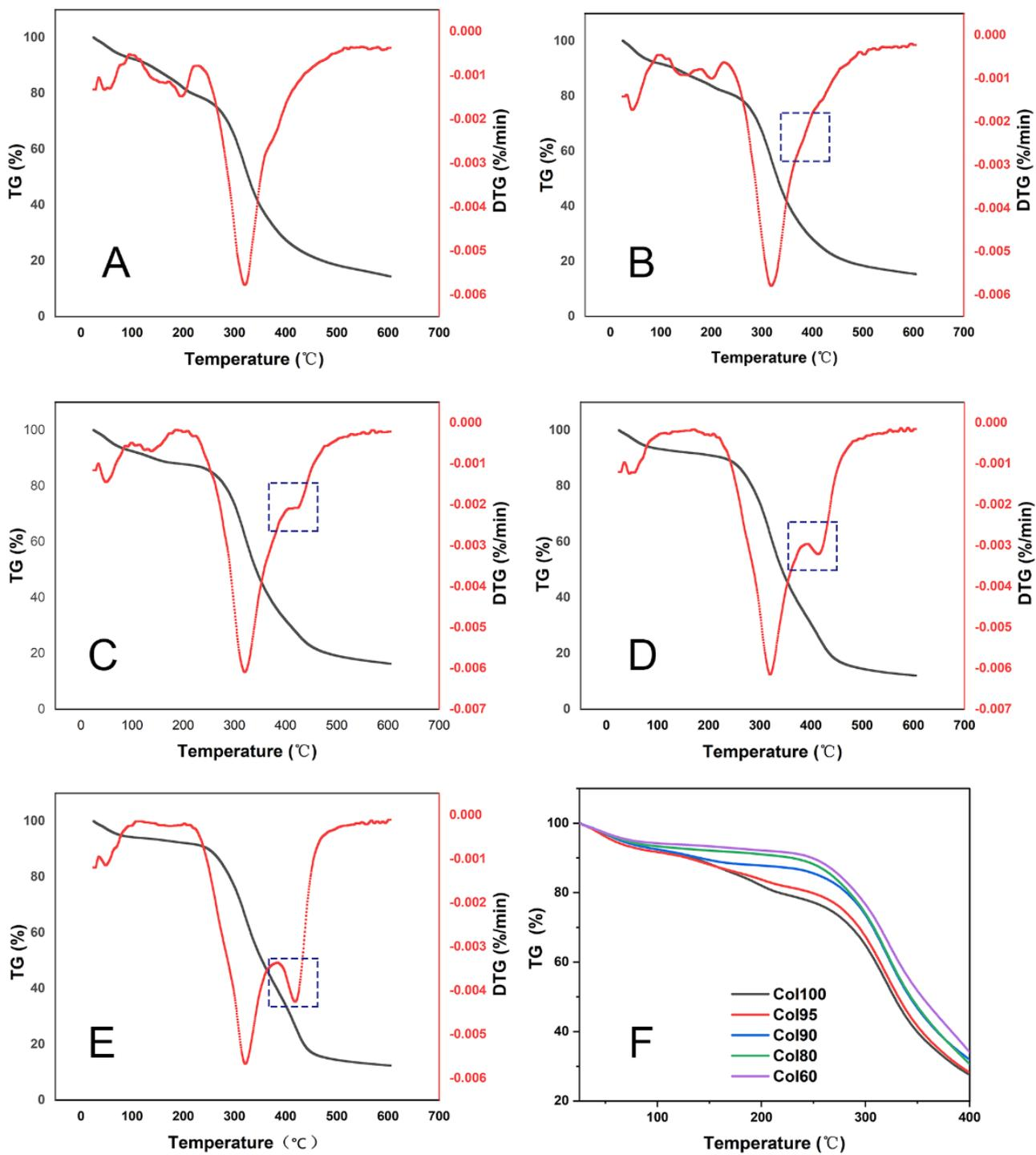
Figure 5. TG-DTA thermogravimetric curve. (A) Col100; (B) Col195; (C) Col190; (D) Col180; (E) Col160; (F) Local enlarged view of TG curve.
