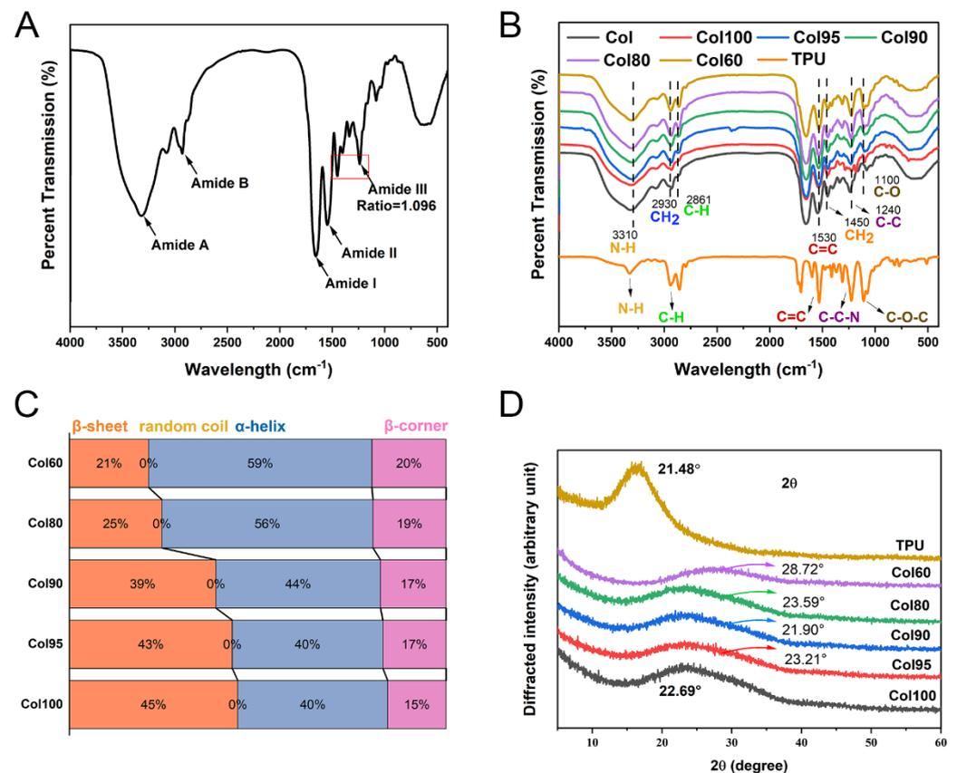
**Figure 3.** Spectroscopy analysis. (A) FTIR of collagen; (B) FTIR of Col-TPU composite nanofiber membranes; (C) Conformation relative content of amide I band in Col-TPU composite nanofiber membranes; (D) XRD of Col-TPU composite nanofiber membranes.
