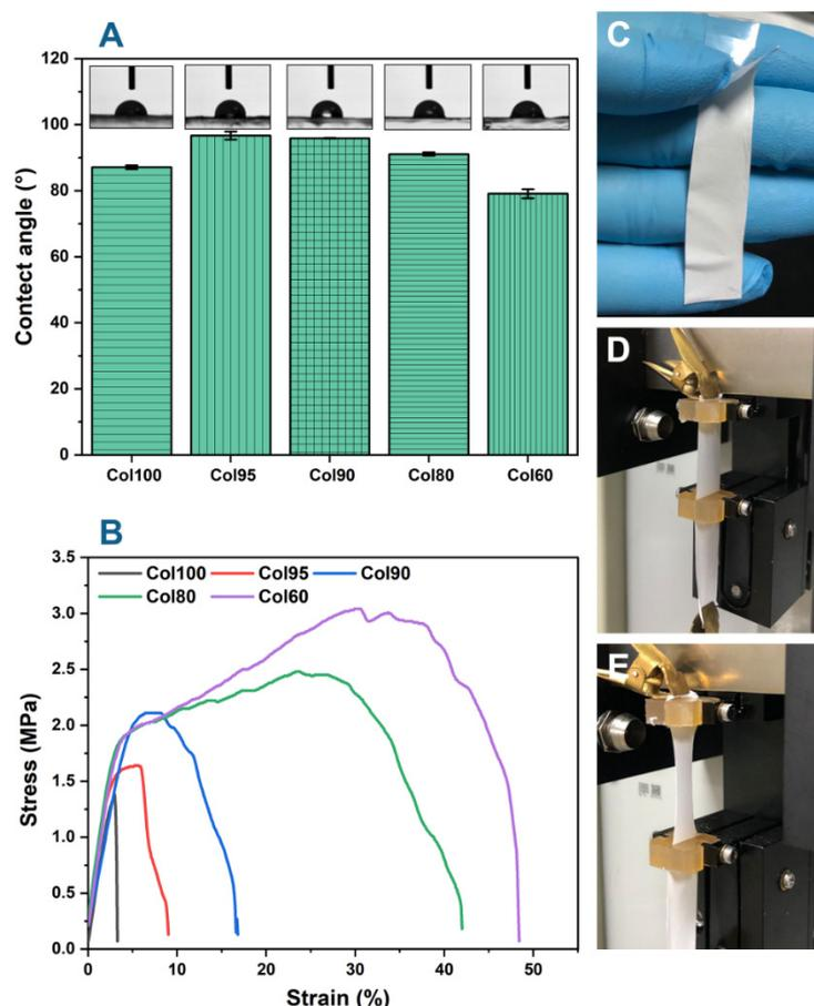
**Figure 6.** Properties of Col based composite nanofiber membranes. (A) WCA; (B) Stress–strain curve; (C) Prepared Col-TPU composite nanofiber membrane; (D) Before tensile test; (E) After tensile test.
