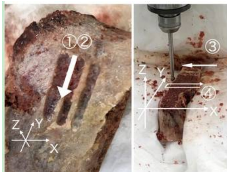
Figure 1. Relationship between the material and the grinding procedure. The left figure is a photograph after manual grinding of the cortex. The photo on the right is the machine procedure. Every series was repeated three times and recorded in the data logger.
