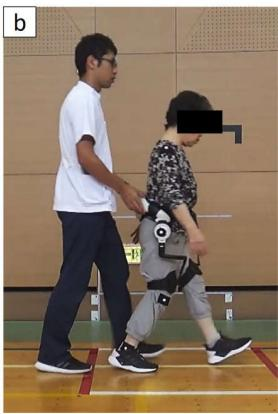
**Figure 1.** (a) The Honda Walking Assistive Device<sup>®</sup> (HWA) and tablet. (b) Gait training with HWA. Motors on the hip joint assist leg movement based on data obtained by the hip angle sensors during walking to improve gait symmetry, lifting a leg from the ground, extending forward during the swing phase, and hip extension to proceed forward in the stance phase.
